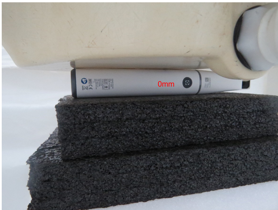
Picture 4: Right Edge, the distance from EUT to the bottom of the Phantom is 0mm
