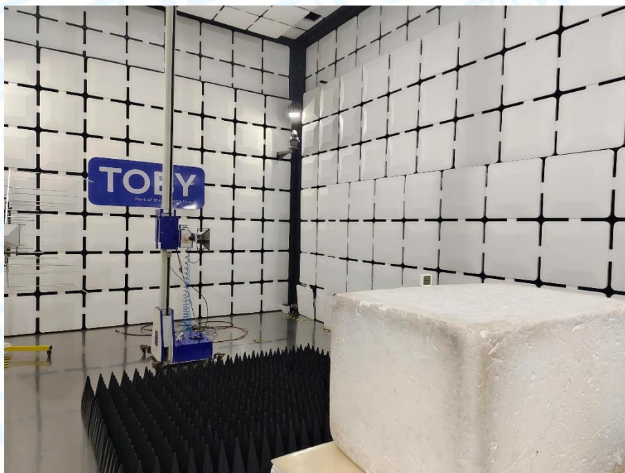
Photo of Setup for Radiated Emission (30MHz~1GHz)
