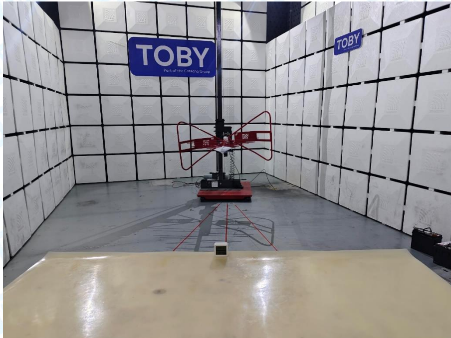
Photo of Setup for Radiated Emission (30MHz~1GHz)
