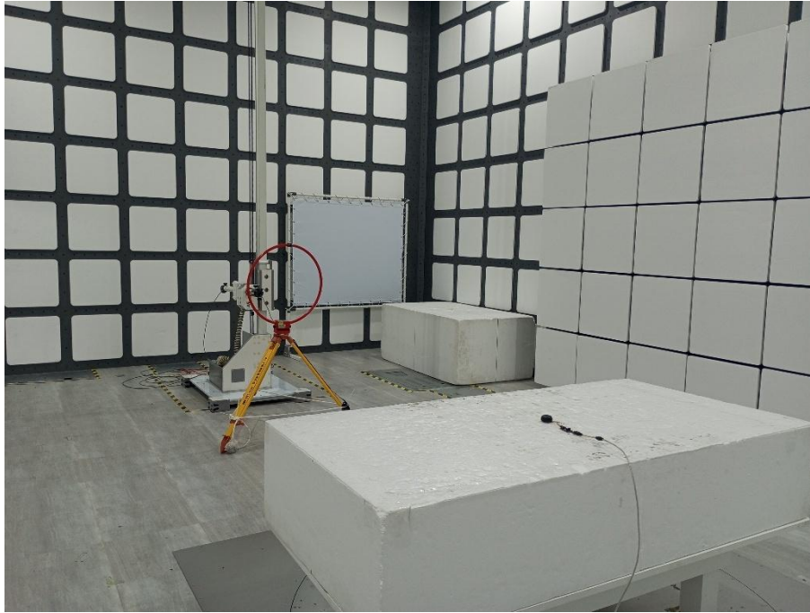
Set-up for Spurious Emissions 9KHz-30MHz Rear View
