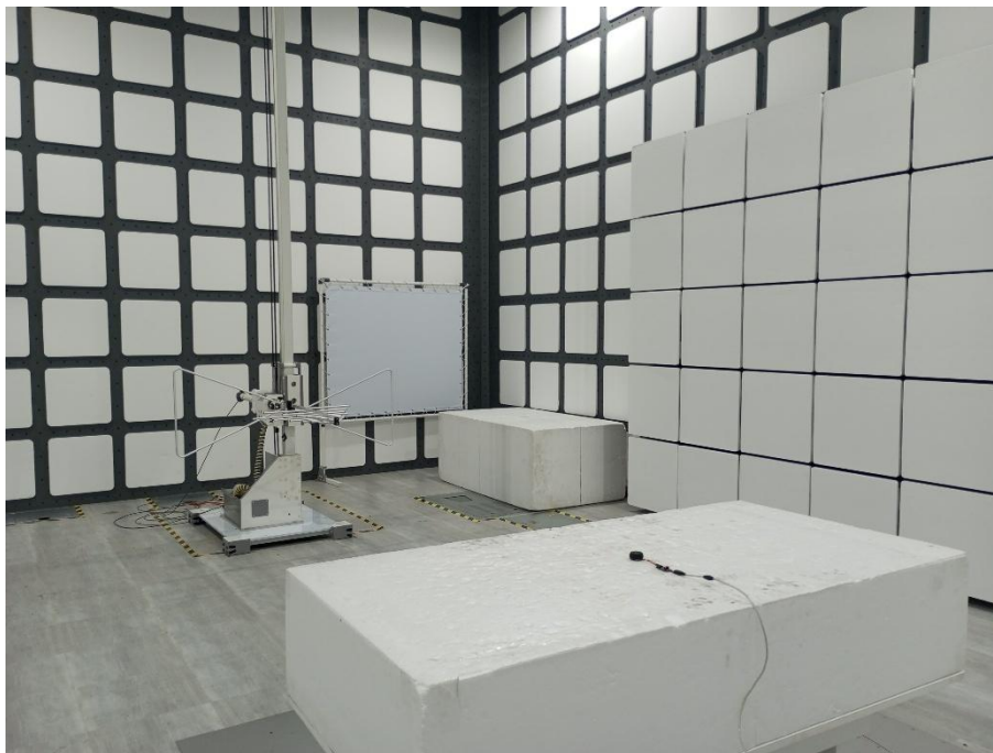
Set-up for Spurious Emissions 30MHz-1000MHz Rear View
