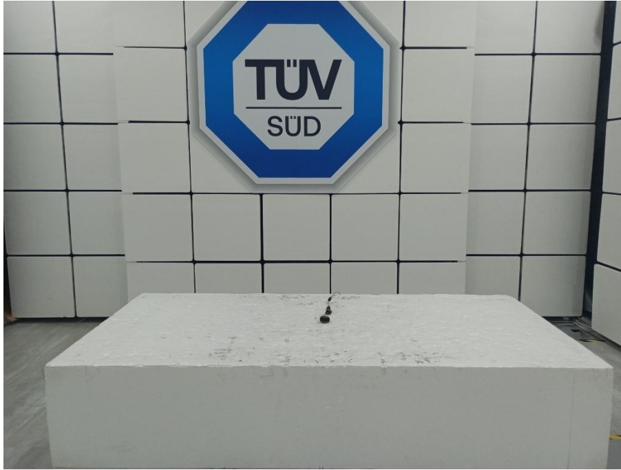
Set-up for Spurious Emissions Front View
