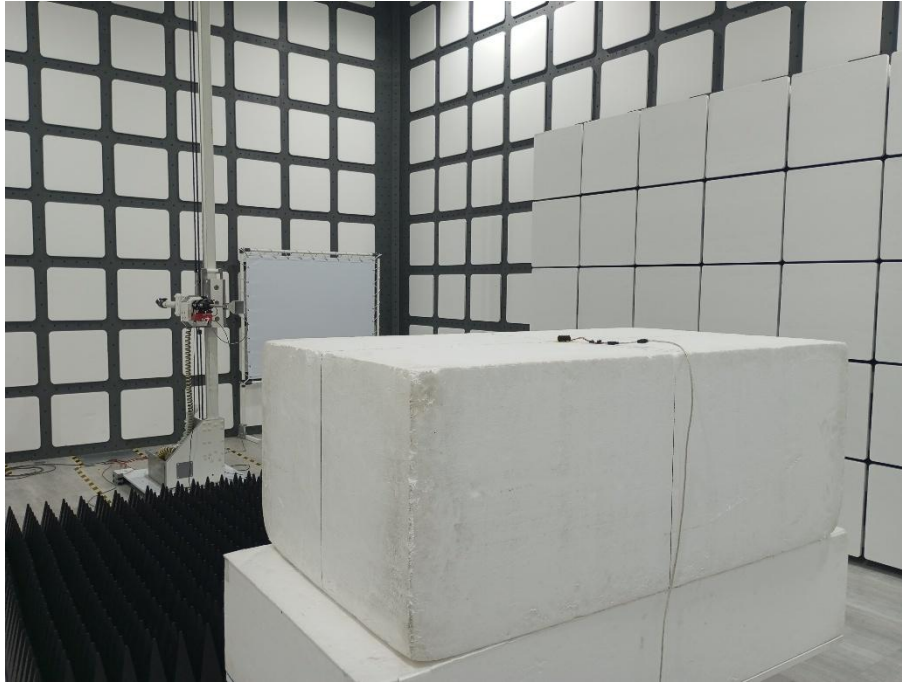
Set-up for Spurious Emissions 18000MHz-25000MHz Rear View
