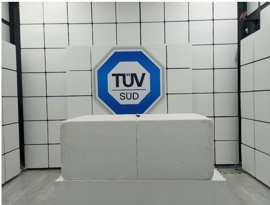
Set-up for Spurious Emissions Front View
