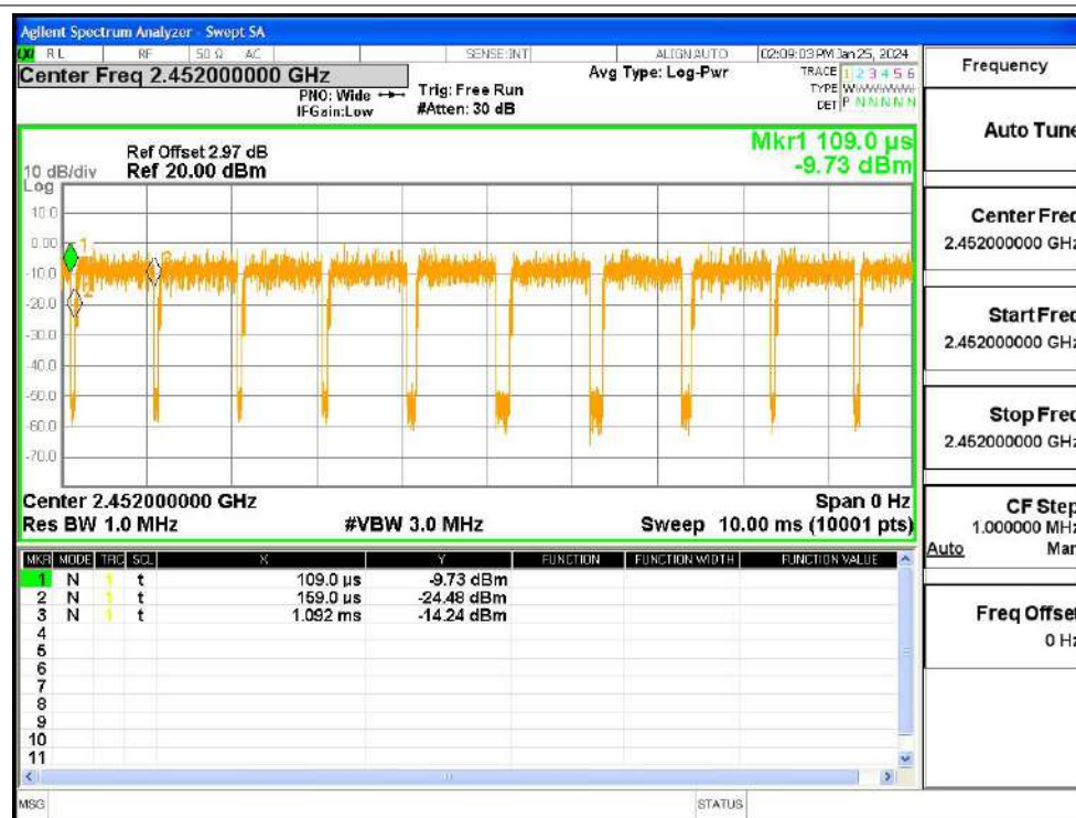
Duty Cycle NVNT n40 2452MHz Ant1
