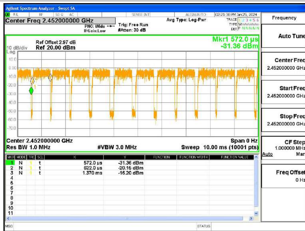
Duty Cycle NVNT ax40 2452MHz Ant1
