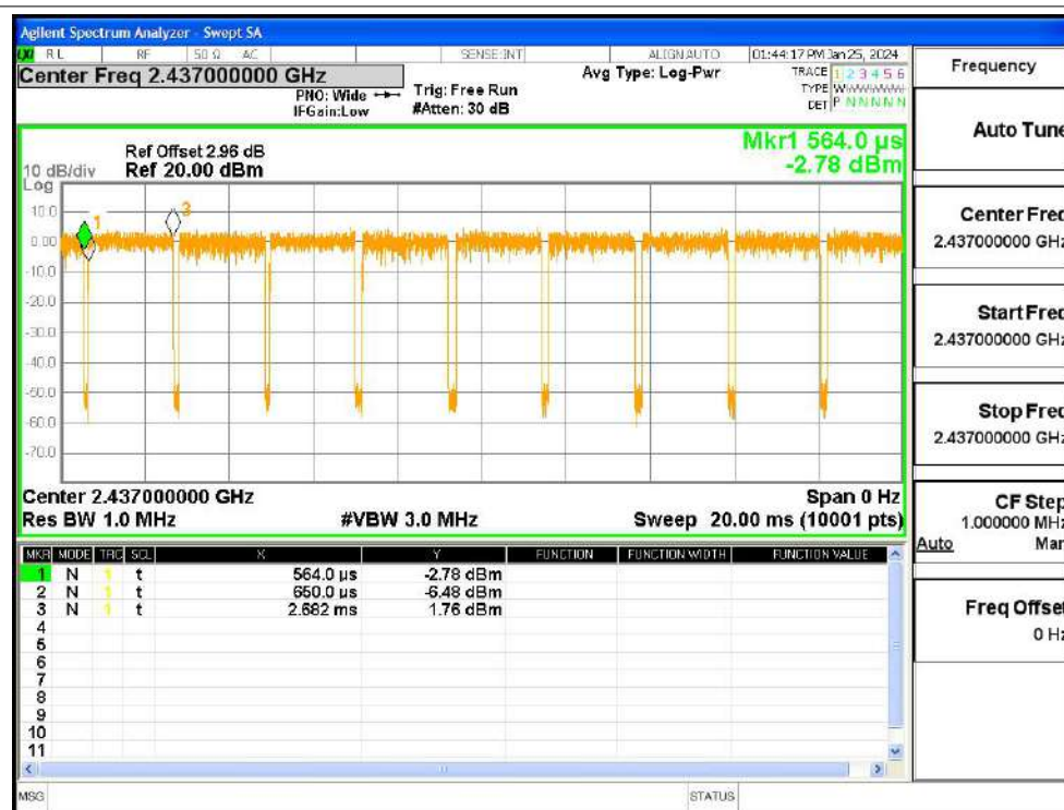
Duty Cycle NVNT g 2462MHz Ant1
