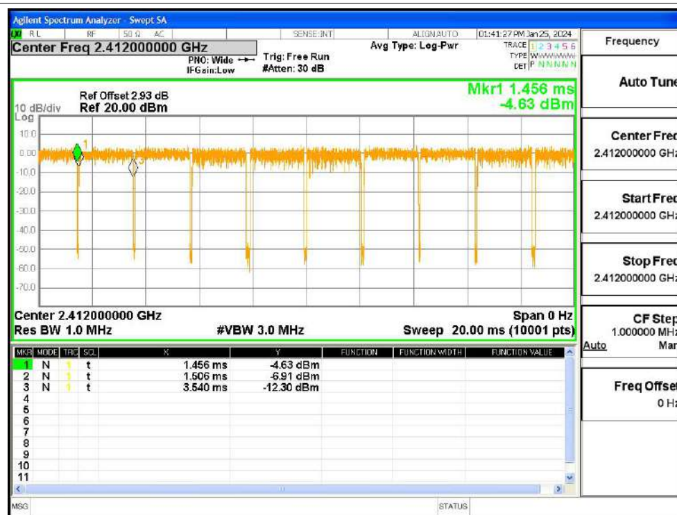
Duty Cycle NVNT g 2412MHz Ant1
