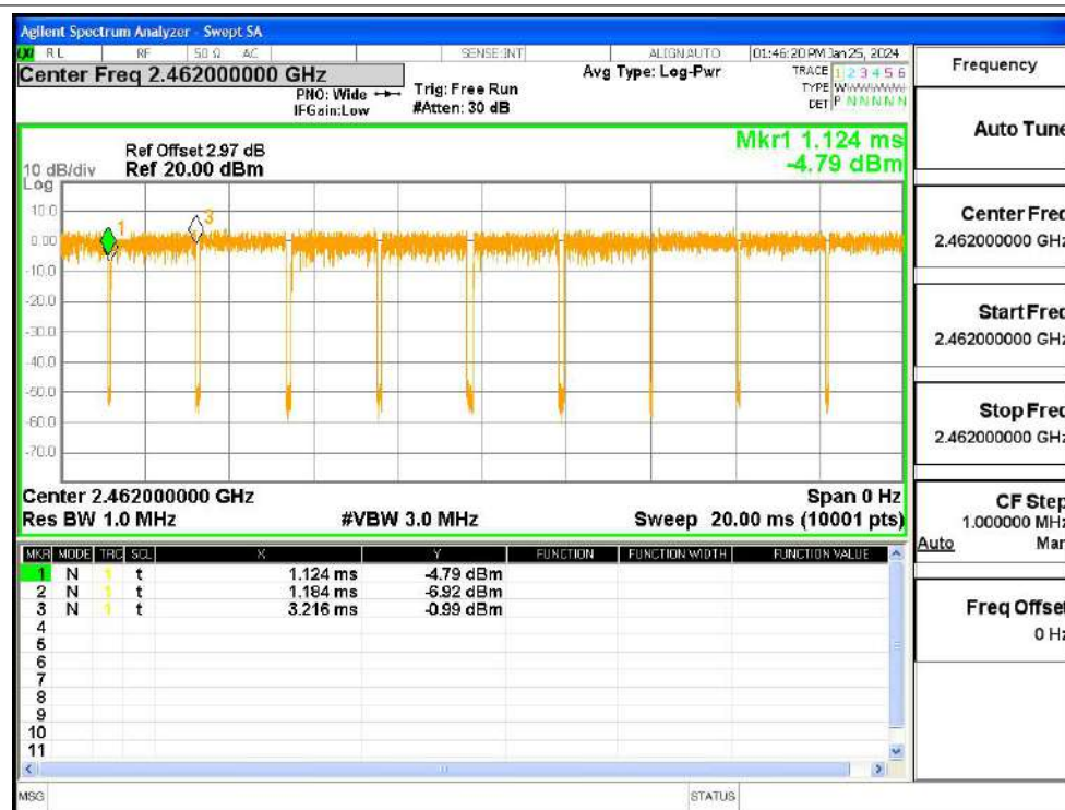
Duty Cycle NVNT g 2462MHz Ant1
