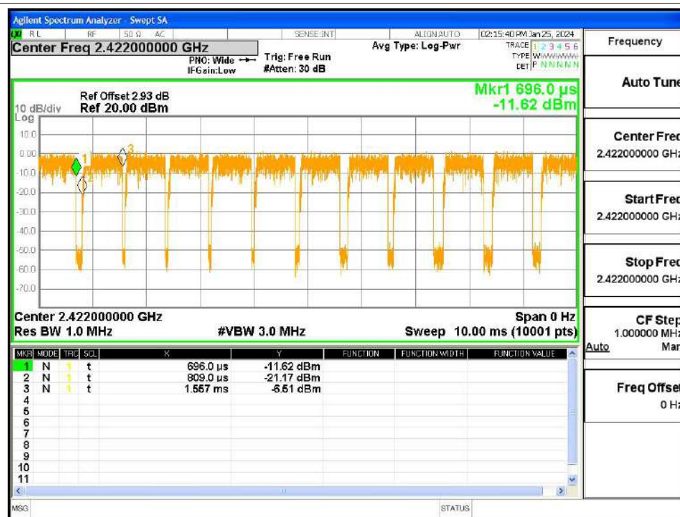
Duty Cycle NVNT ax40 2422MHz Ant1
