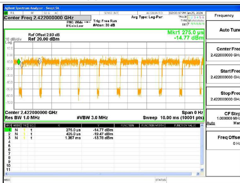
Duty Cycle NVNT n40 2422MHz Ant1
