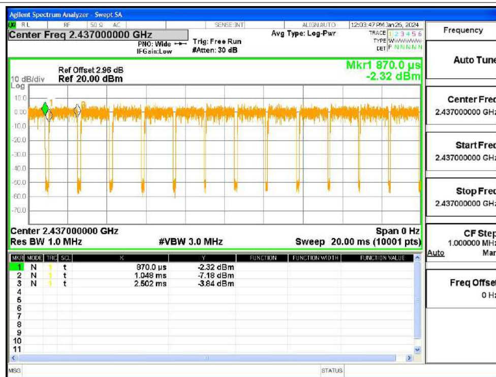
Duty Cycle NVNT ax20 2437MHz Ant1
