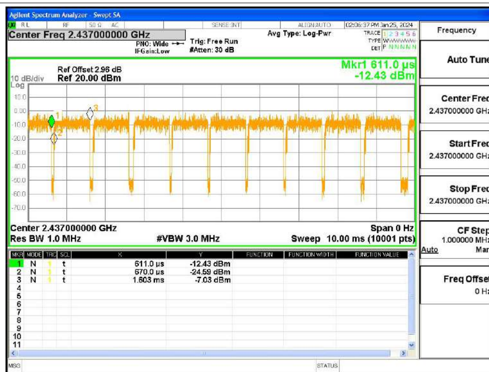
Duty Cycle NVNT n40 2452MHz Ant1
