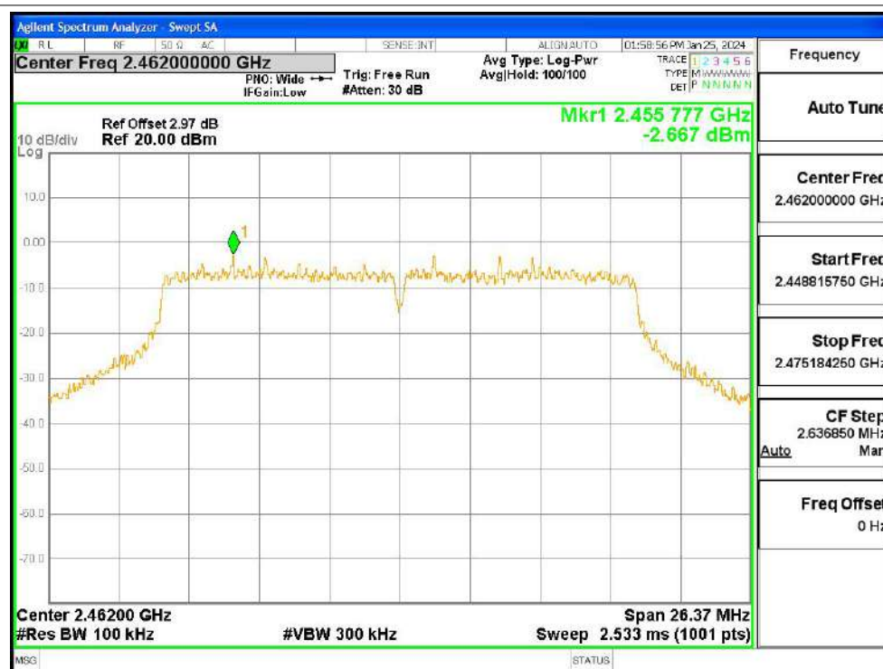
PSD NVNT n40 2422MHz Ant1
