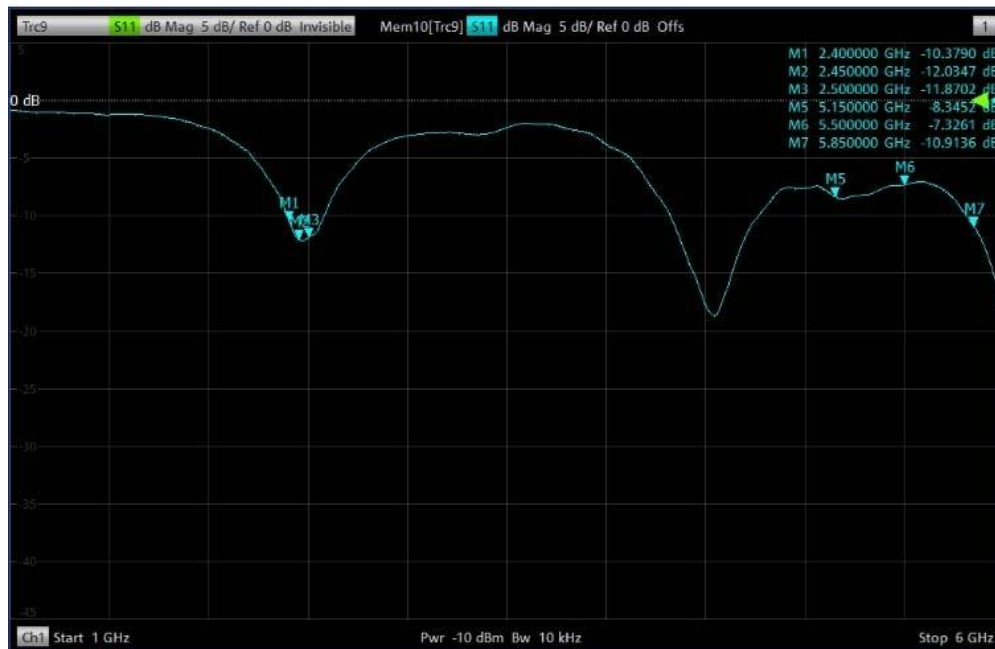
Figure 2 ECG Bluetooth Antenna Return Loss
