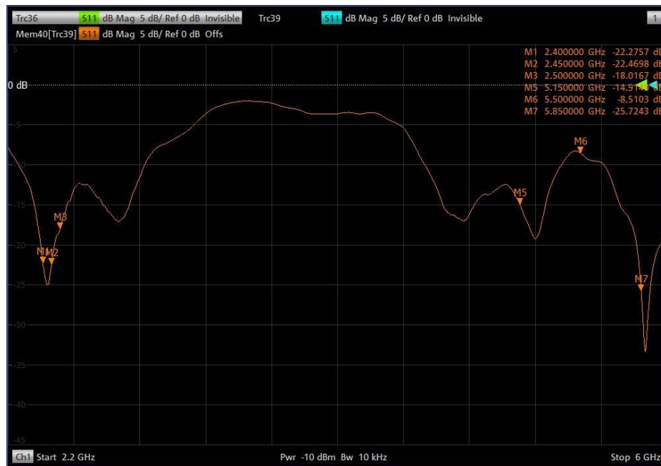
Figure 2 Wi-Fi Antenna Return Loss
