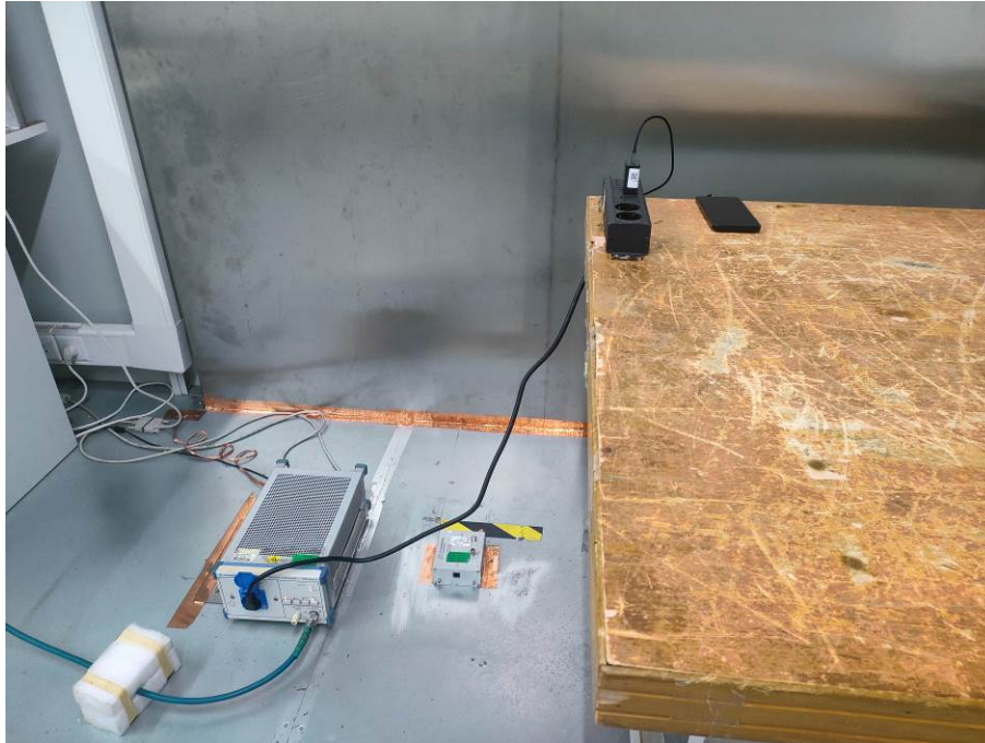
Conducted Emissions - Front View
