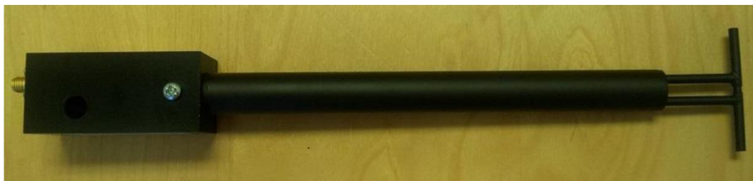
Figure 1 – MVG COMOSAR Validation Dipole
