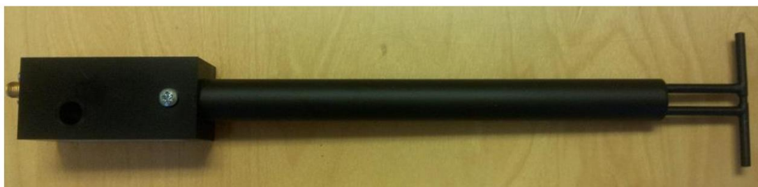
Figure 1 – MVG COMOSAR Validation Dipole
