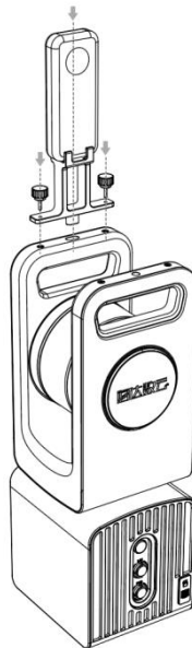
Figure 3-2.3 Installation diagram of HD TLS360 system camera
