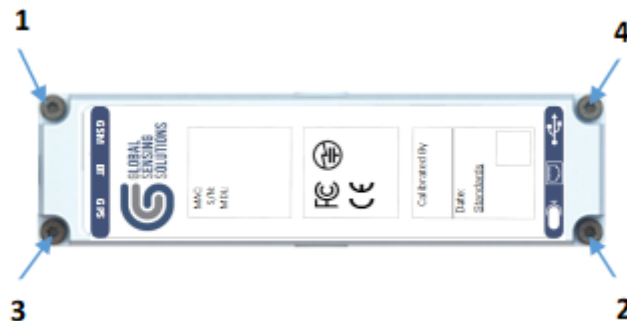
Figure 4 – Top Case Screw Removal Sequence
