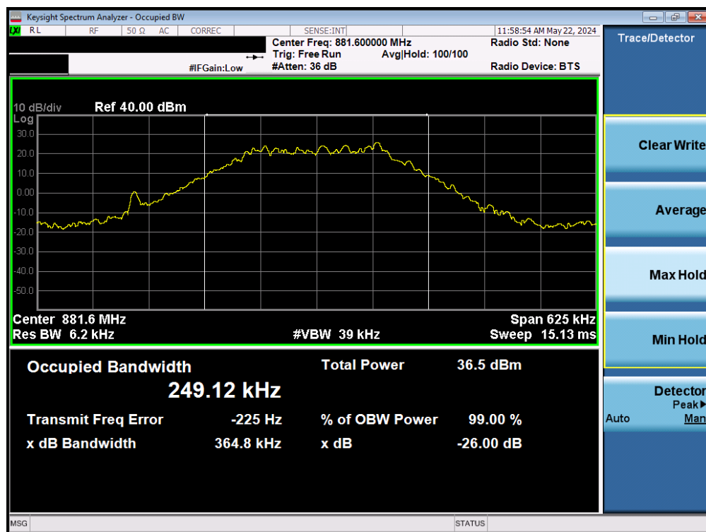
Plot 7-12. Conducted Power Output Data (GSM 850)
