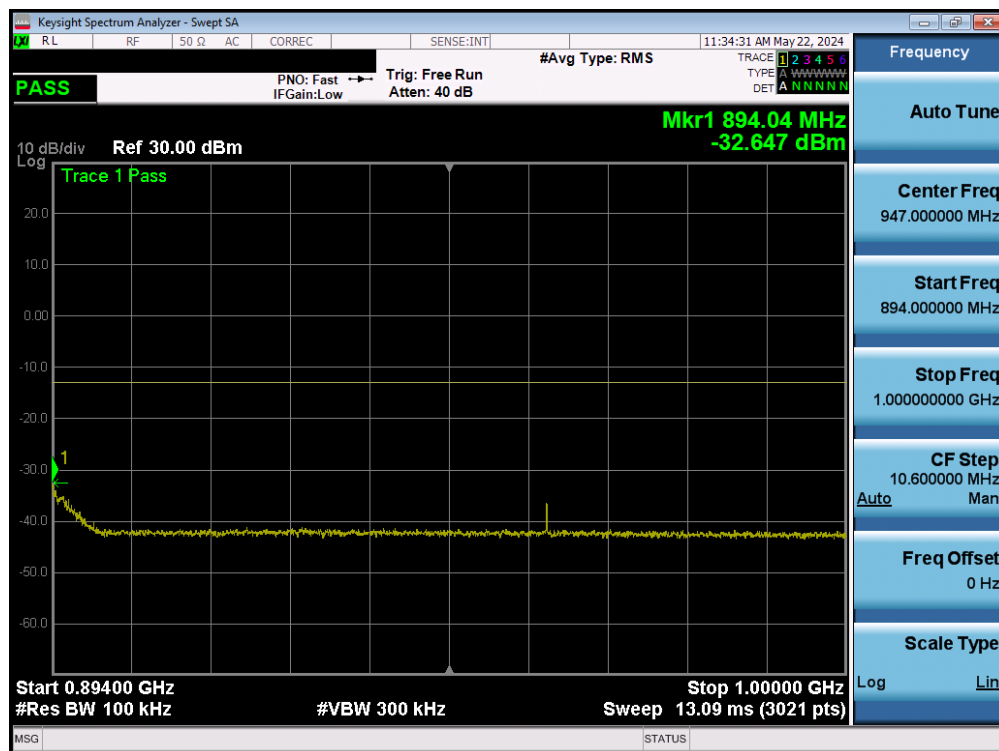
Plot 7-17. Conducted Spurious Plot (LTE Band 26/5 – Mid Channel)
