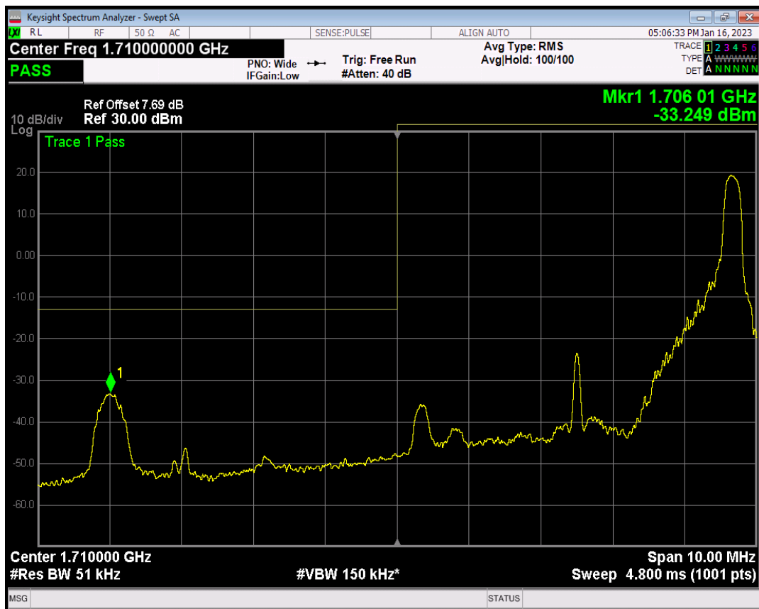
Band4 QPSK BW=5MHz Channel=19975 RB Size=25 Position=#0
