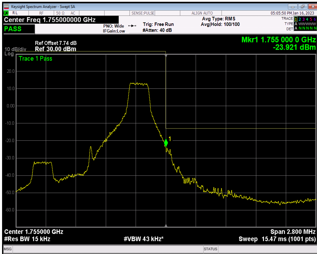
Band4 QAM16 BW=1.4MHz Channel=20393 RB Size=6 Position=#0
