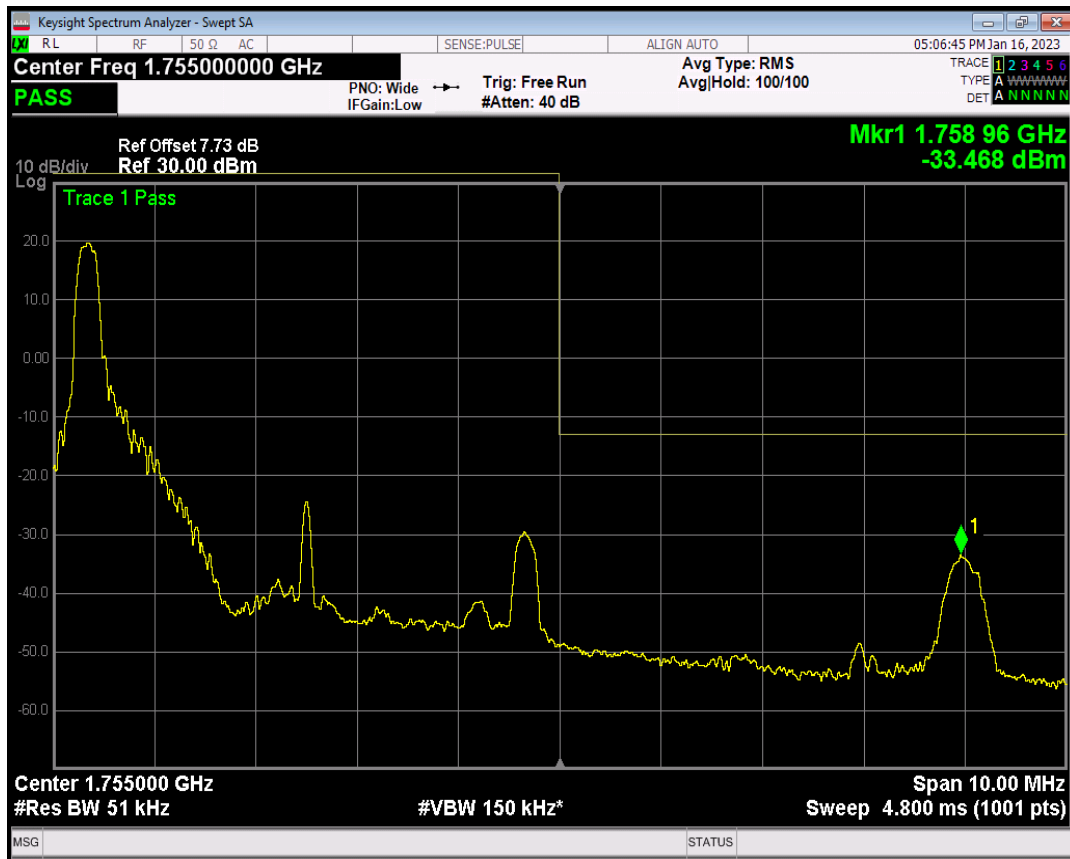
Band4 QPSK BW=5MHz Channel=20375 RB Size=1 Position=#Max
