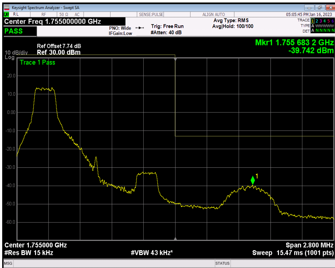
Band4 QAM16 BW=1.4MHz Channel=20393 RB Size=1 Position=#Max
