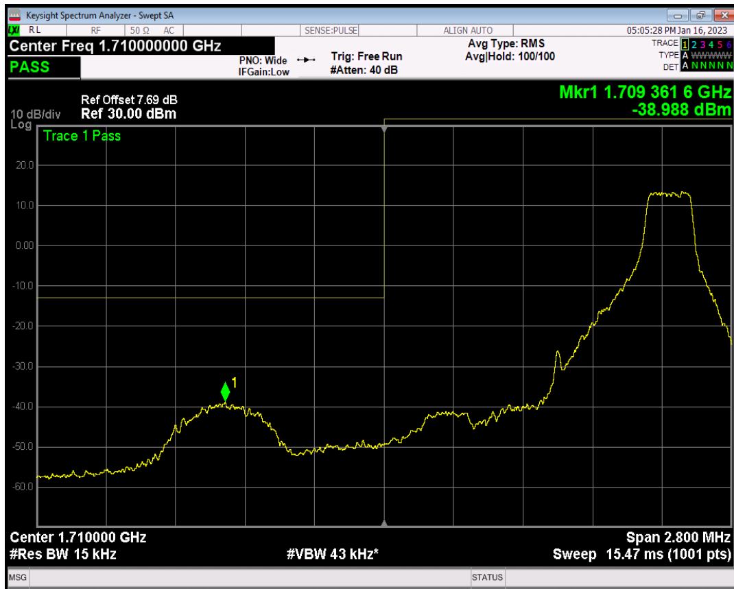
Band4 QAM16 BW=1.4MHz Channel=19957 RB Size=6 Position=#0
