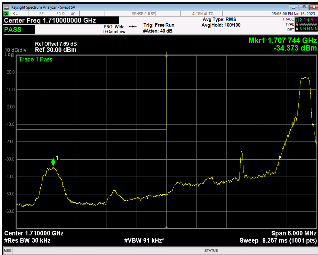
Band4 QPSK BW=3MHz Channel=19965 RB Size=15 Position=#0
