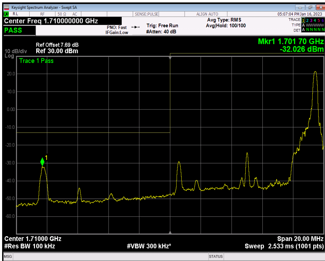
Band4 QPSK BW=10MHz Channel=20000 RB Size=50 Position=#0
