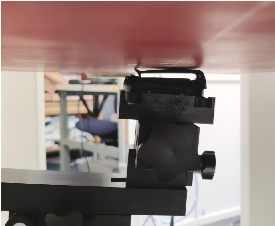
Figure 8 Back side with belt-clip against the phantom, 0mm separation distance
