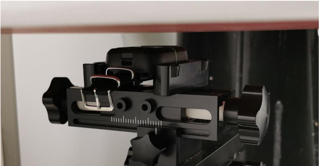
Figure 10 Front side of the DUT with wristband against the phantom, 10mm separation distance, next-to-mouth position.
