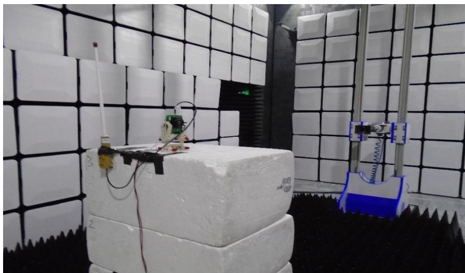
Figure 49 – Whip Z Plane, 1GHz to 5GHz
