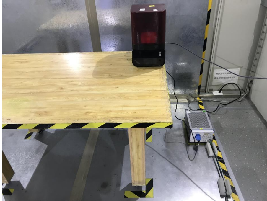
Conducted Emissions (Left View)
