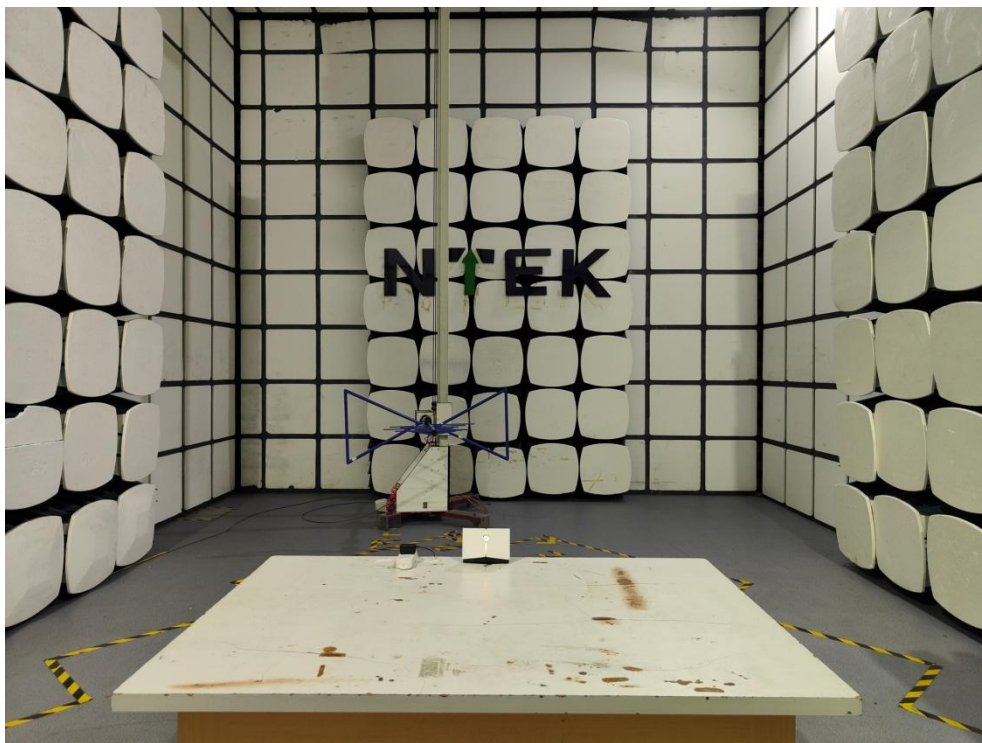
Radiated Measurement Photos(30MHz~1GHz )
