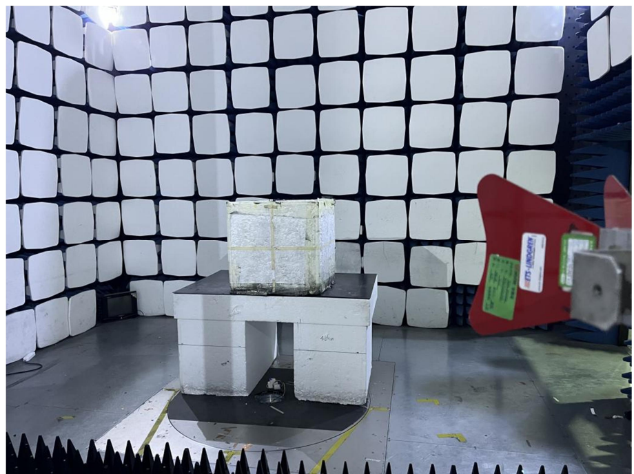
Radiation Emission Test Setup (1GHz to 18GHz)
