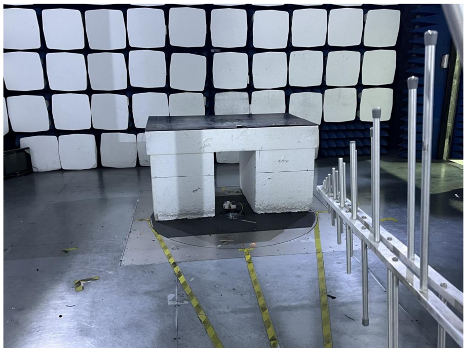
Radiation Emission Test Setup (30MHz to 1GHz)
