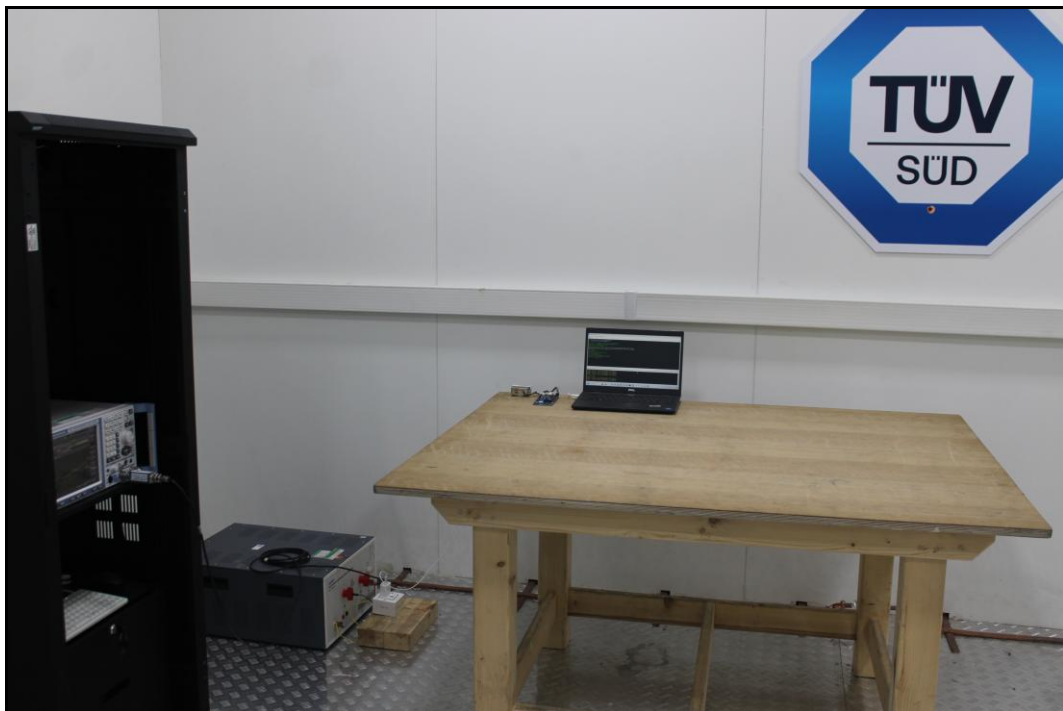
Conducted AC Power Lines Test Setup
