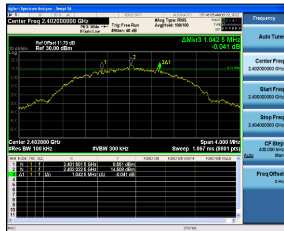
6dB Occupied Bandwidth Mode 2 CH00 (2402MHz)
