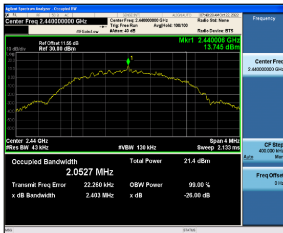
99% Occupied Bandwidth Mode 2 CH19 (2440MHz)
