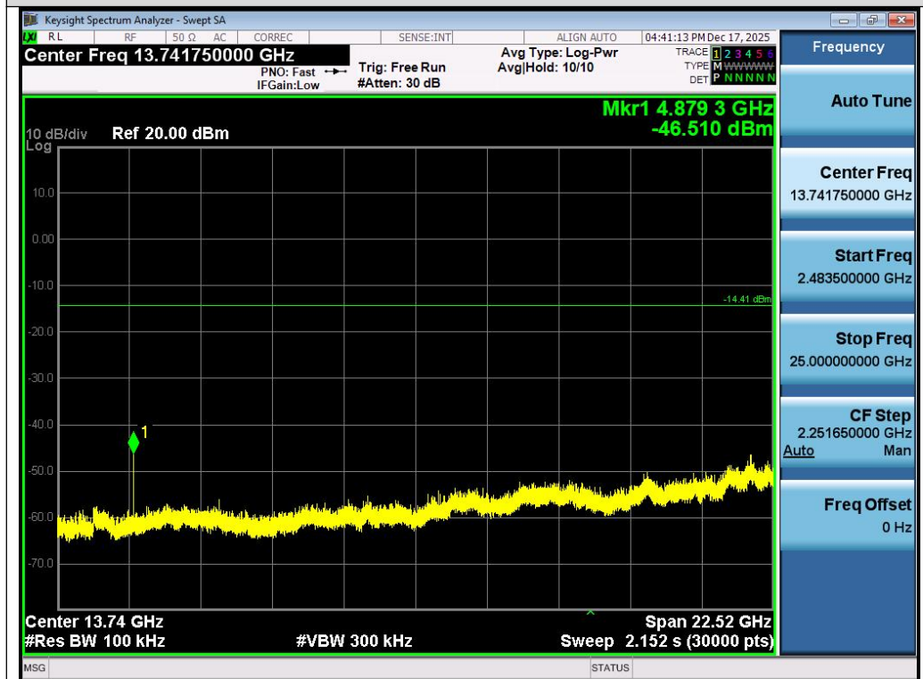
Test_Graph_LE1M_ANT1_2440_1Mbps_Higher Band Emissions
