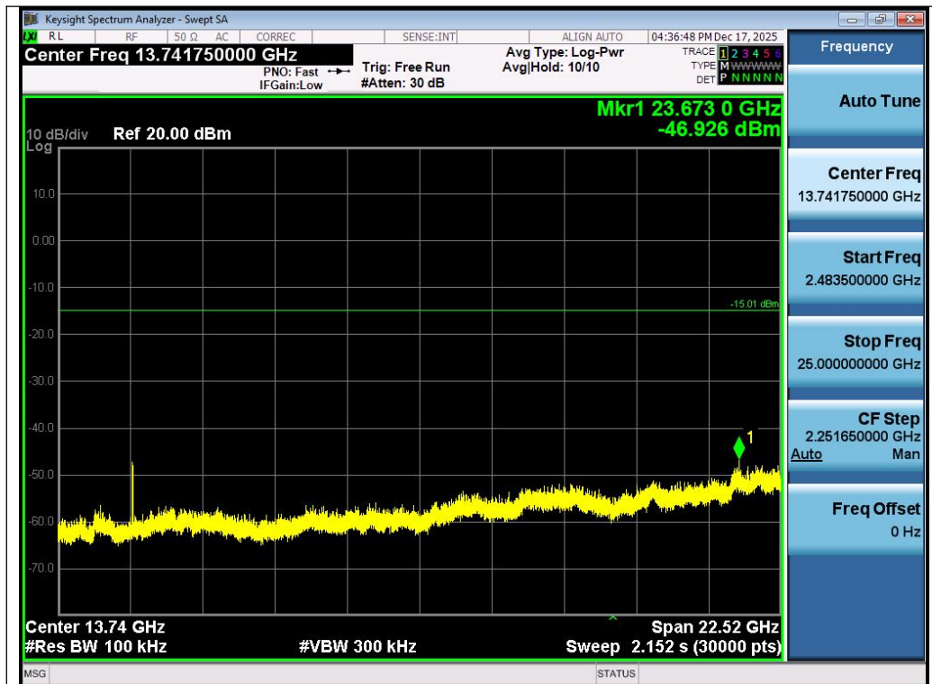
Test_Graph_LE1M_ANT1_2402_1Mbps_Higher Band Emissions
