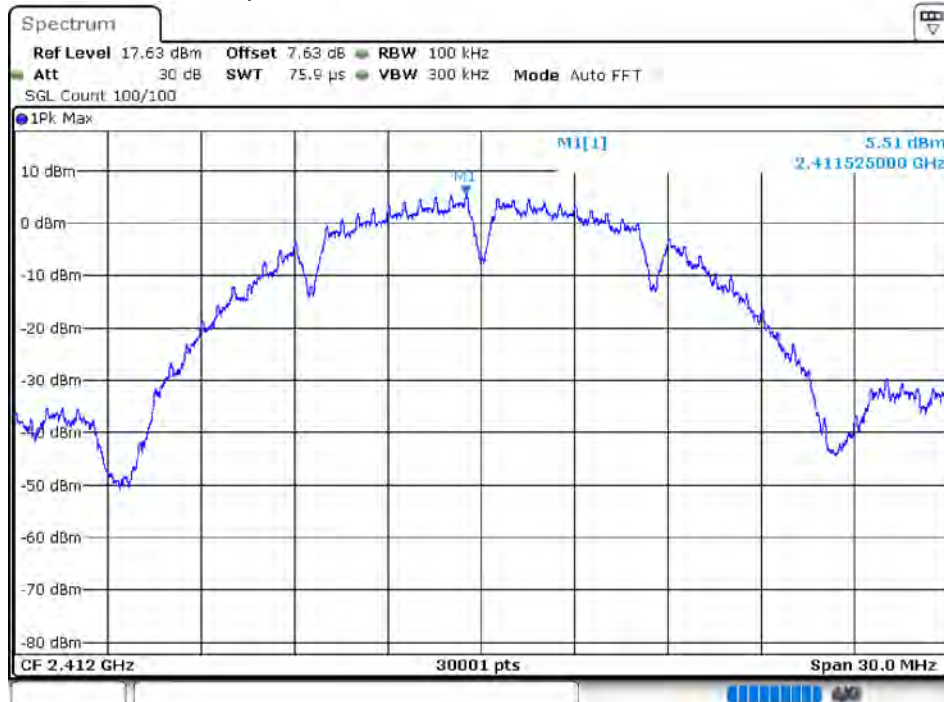
Tx. Spurious NVNT 802.11b 2412MHz Ant 1 Ref
