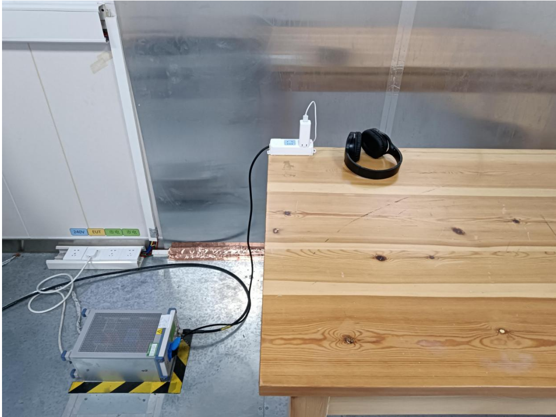
Conducted emission test setup
