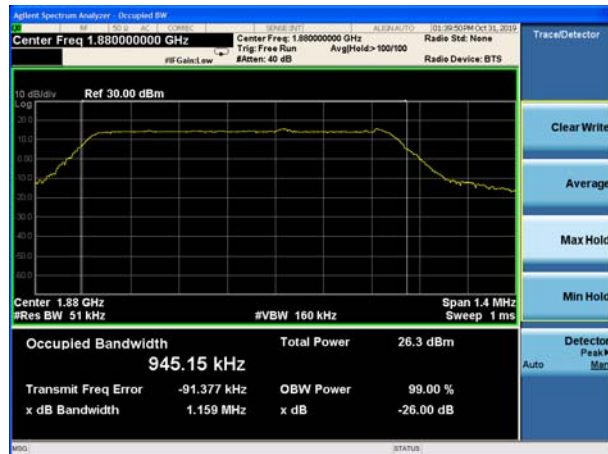
LTE Band 2 5MHz 16QAM CH-Middle
