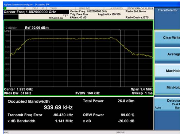
LTE Band 25 5MHz 16QAM CH-Middle
