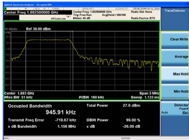
LTE Band 25 10MHz 16QAM CH-Middle
