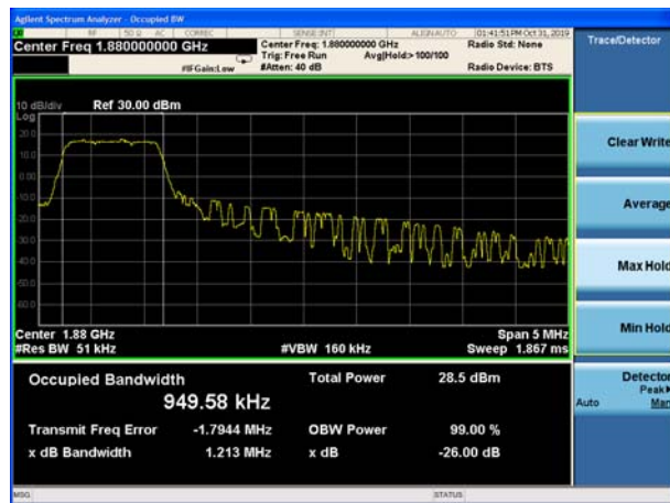
LTE Band 2 15MHz 16QAM CH-Middle
