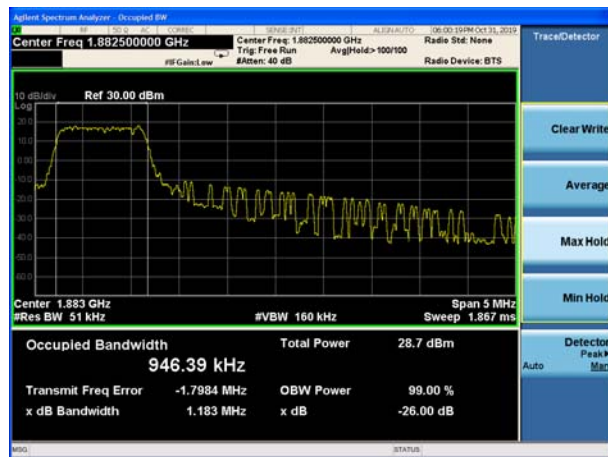
LTE Band 25 15MHz 16QAM CH-Middle
