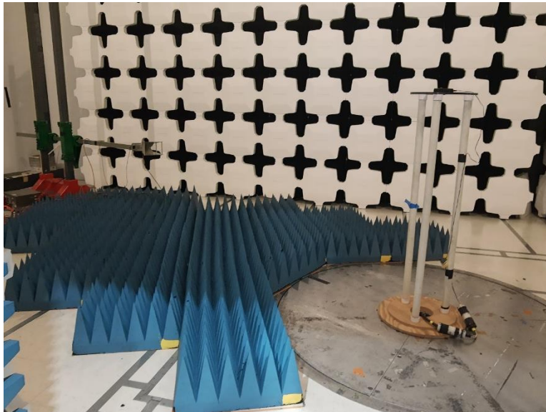
Photograph 4. Radiated Emissions - 1-18GHz Test Setup
