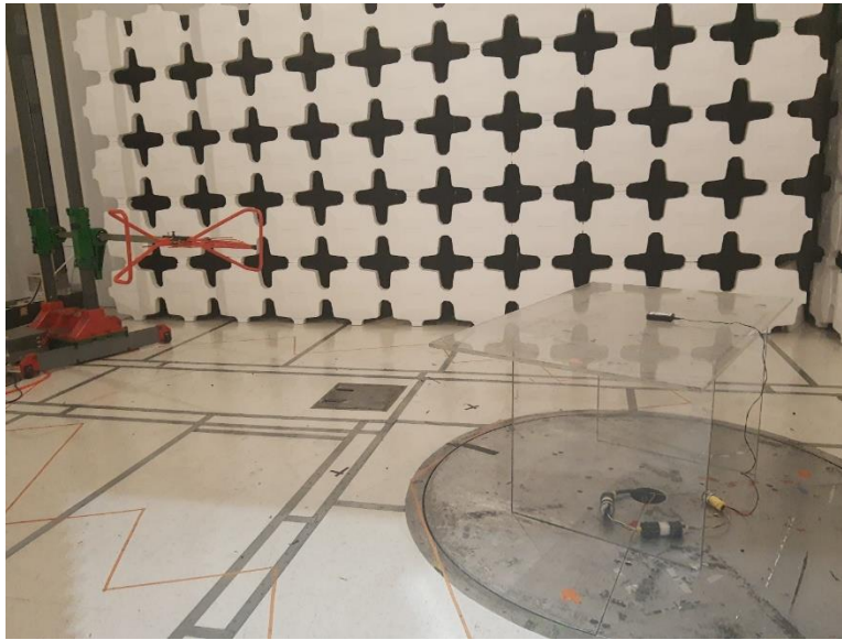
Photograph 3. Radiated Emissions - 30-1000MHz Test Setup
