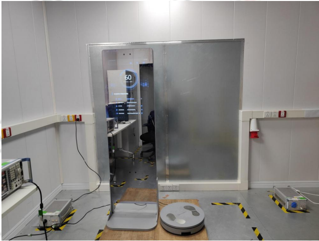
Radiated Emissions for 30MHz~1GHz
