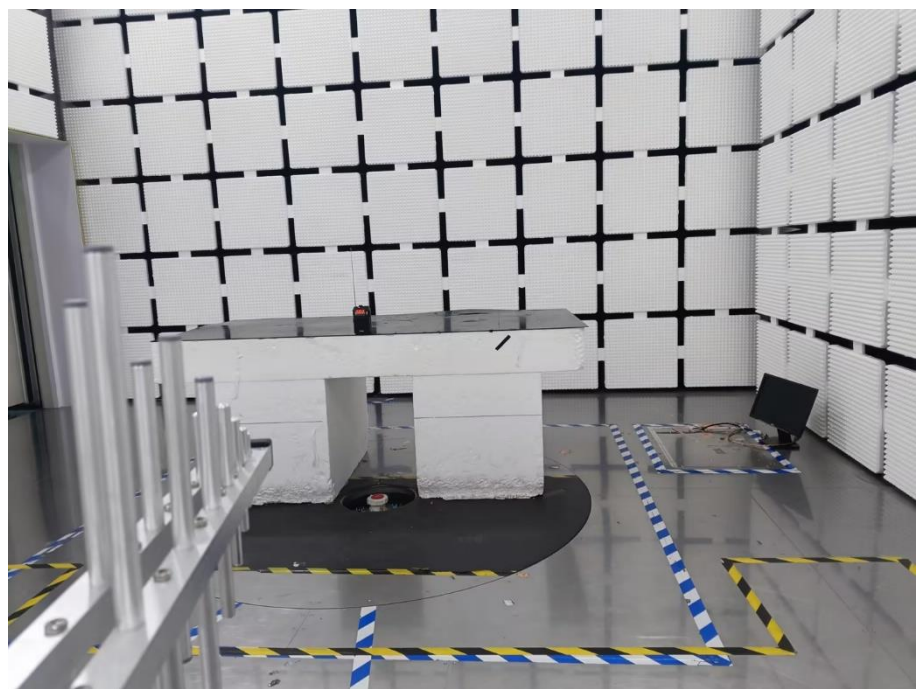
Radiation Emission Test Setup (30MHz to 1GHz)
