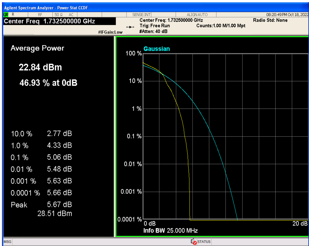
Band41 QPSK BW=5MHz Channel=40620 RB Size=1 Position=#0
