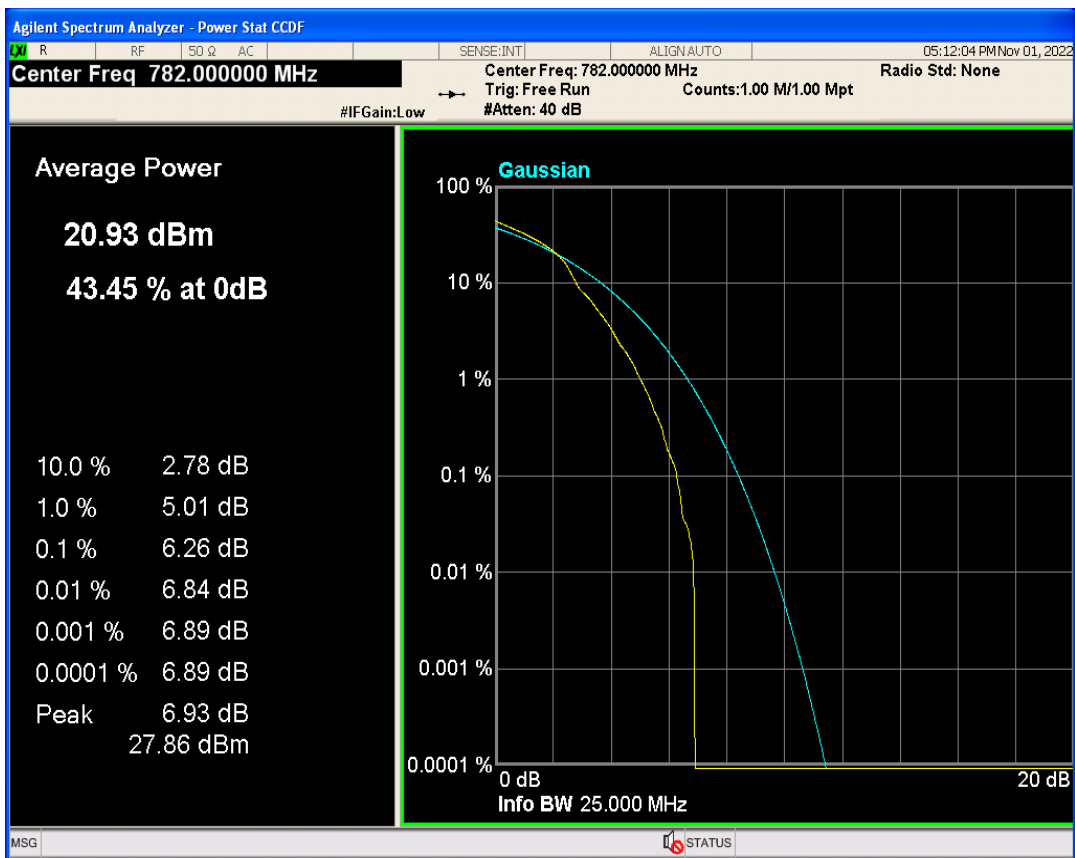
Band13 QPSK BW=10MHz Channel=23230 RB Size=1 Position=#0
