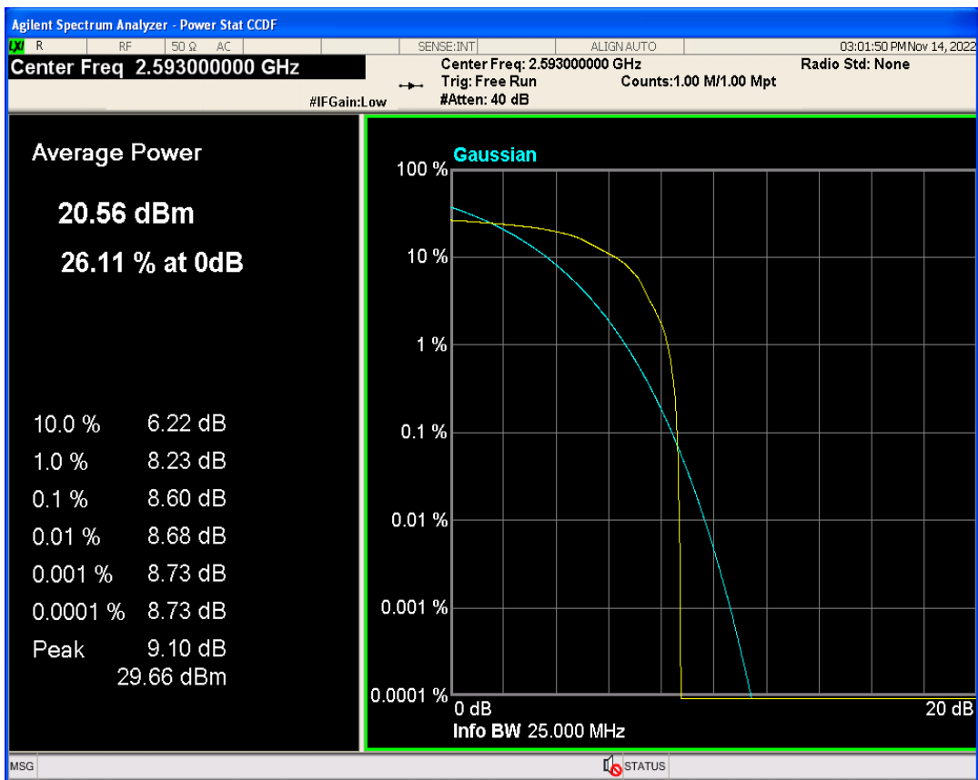
Band41 QPSK BW=10MHz Channel=40620 RB Size=1 Position=#0
