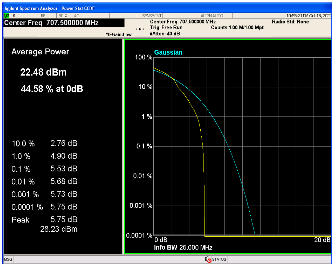
Band12 QPSK BW=10MHz Channel=23095 RB Size=1 Position=#0
