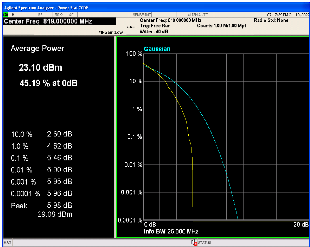
Band26a QAM16 BW=3MHz Channel=26740 RB Size=1 Position=#0
