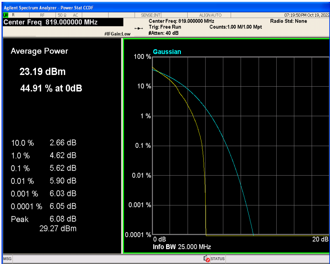
Band26a QAM16 BW=10MHz Channel=26740 RB Size=1 Position=#0
