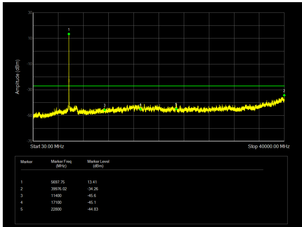
Tx. Spurious NVNT 802.11ac40 5510MHz Ant1 Emission
