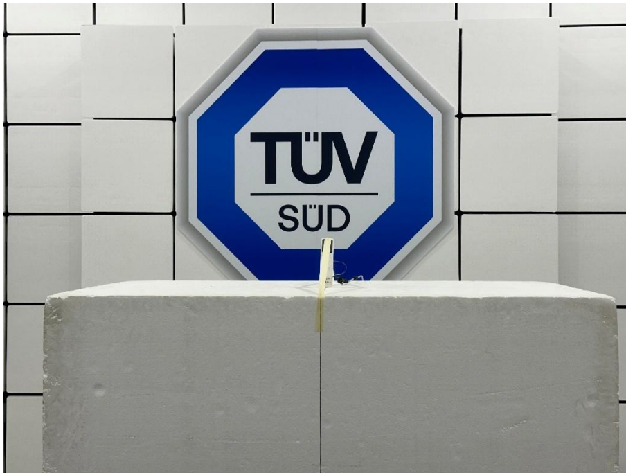
Set-up for Spurious Emissions (Rear View)
