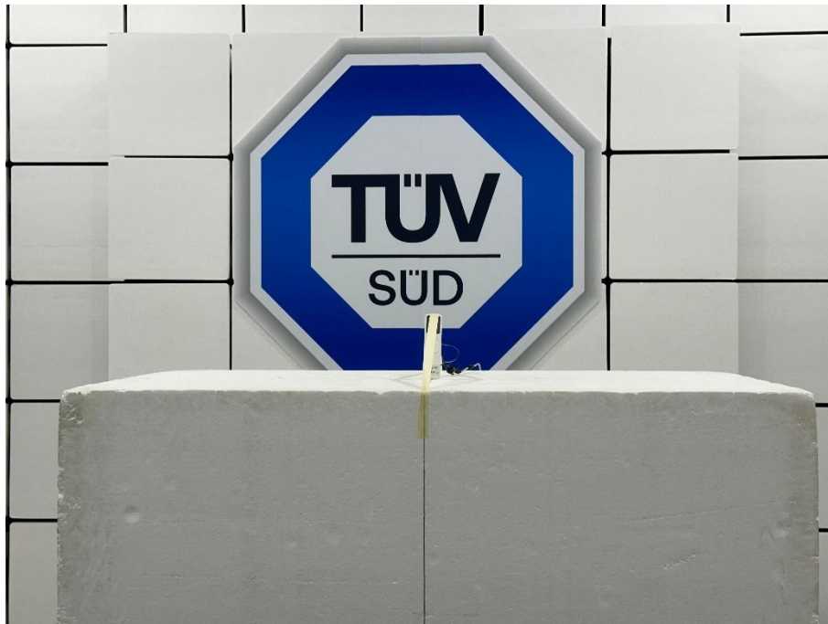
Set-up for Spurious Emissions (Rear View)
