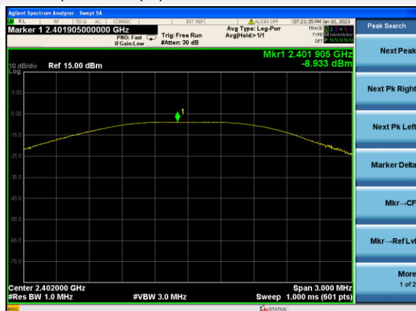
GFSK (BLE 1Mbps) LOW CHANNEL
