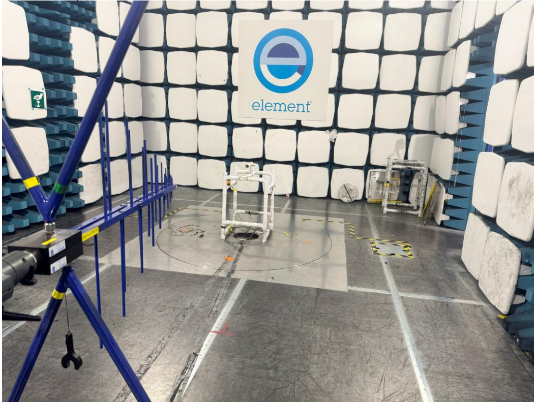
Radiated Spurious Emissions > 1GHz – Handheld:
