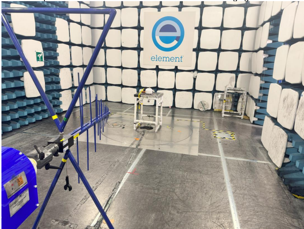
Radiated Spurious Emissions > 1GHz – Hub / Handheld Charging in Hub:
