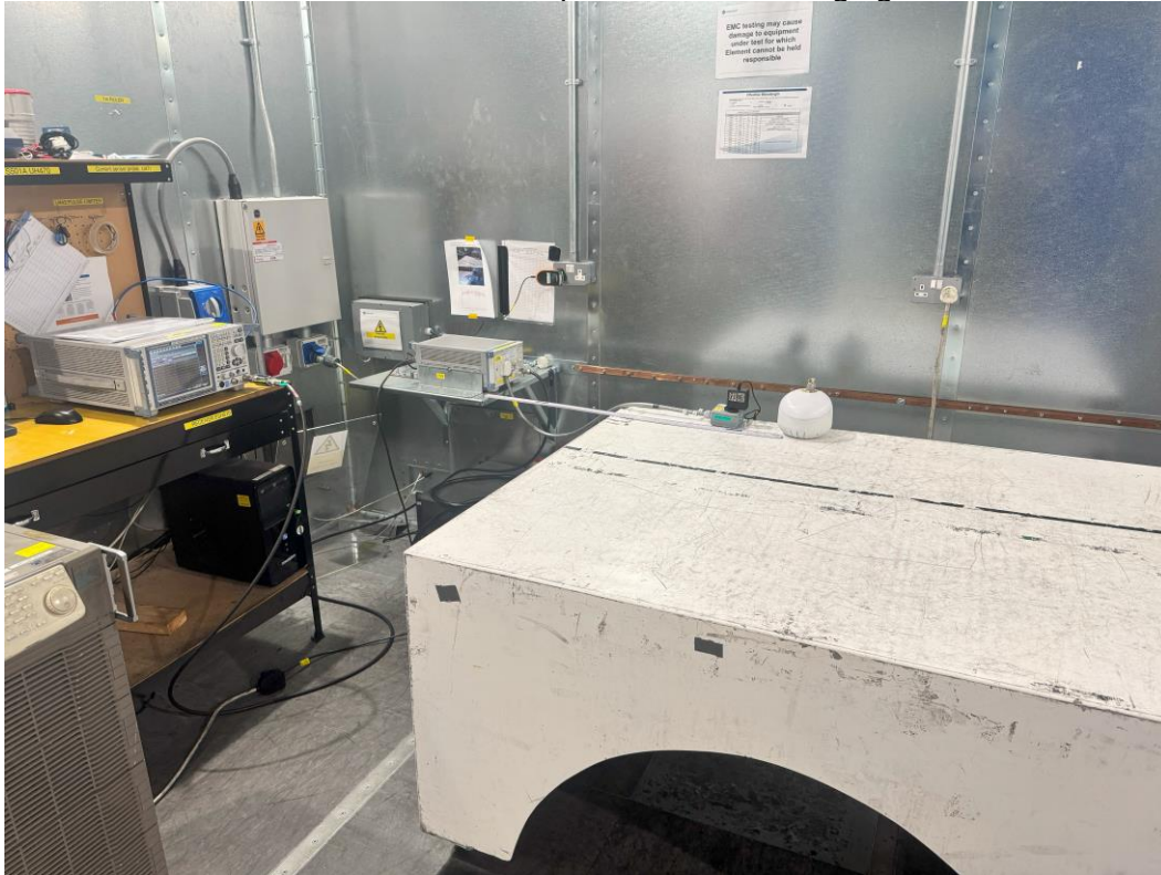
Close up view of Handheld in Radiated Spurious Tests:
