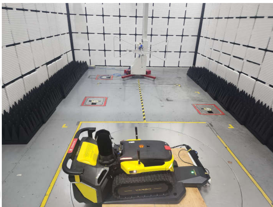
Radiated Emissions Test Setup (30MHz-1GHz)
