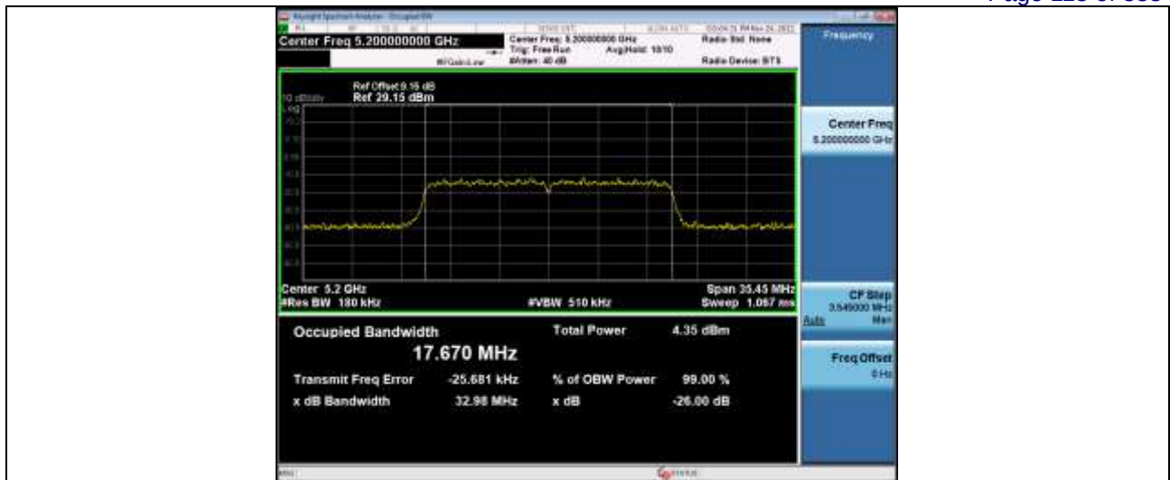
-26dB and 99% Emission Bandwidth 5_2GWiFi_NVNT_ANT5_802_11ac(VHT20)_5240_20M
