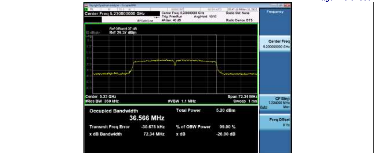
-26dB and 99% Emission Bandwidth 5 2GWiFi NVNT ANT4 802 11ac(VHT80) 5210 80M
