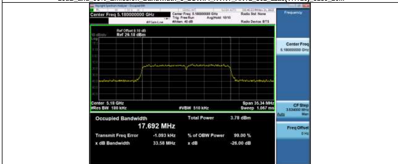
-26dB and 99% Emission Bandwidth 5_2GWiFi_NVNT_ANT2_802_11ac(VHT20)_5180_20M
