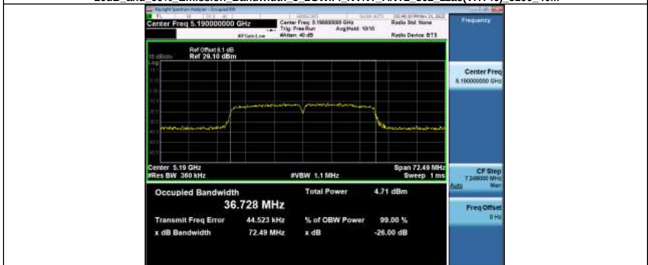
-26dB and 99% Emission Bandwidth 5 2GWiFi_NVNT_ANT2_802_11ac(VHT40)_5190_40M
