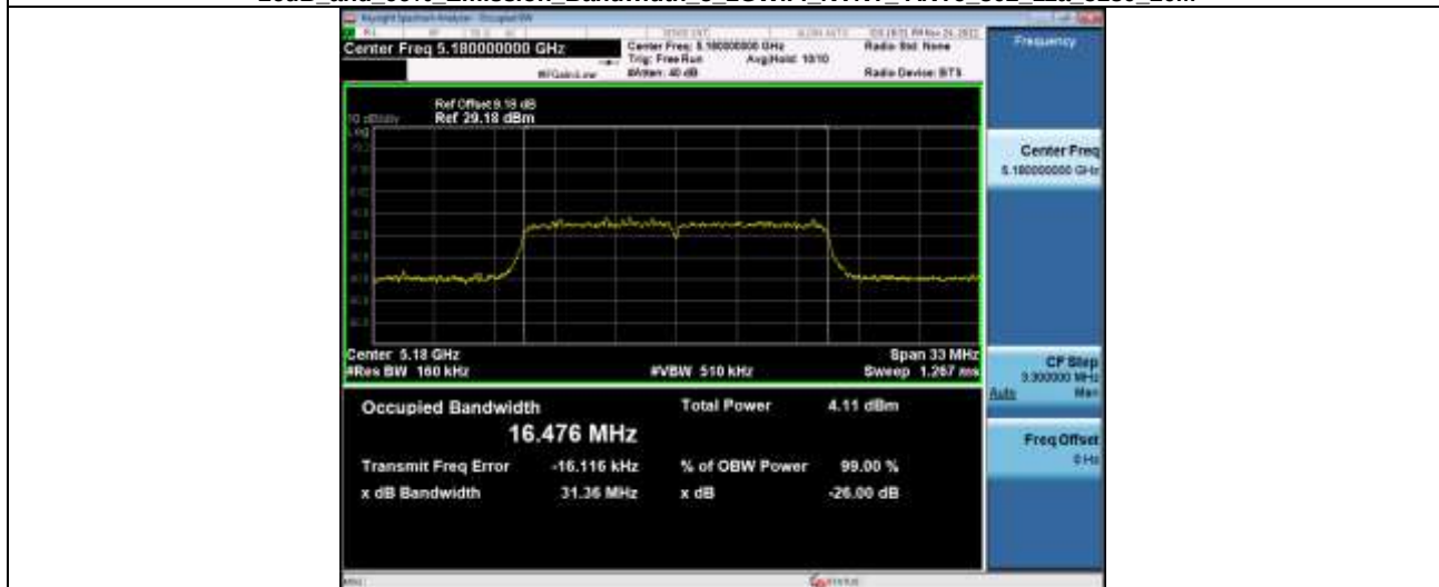
-26dB and 99% Emission Bandwidth 5 2GWiFi NVNT ANT6 802 11a 5180 20M
