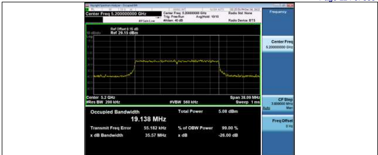
-26dB and 99% Emission Bandwidth 5_2GWiFi_NVNT_ANT4_802_11ax(HE20)_5240_20M
