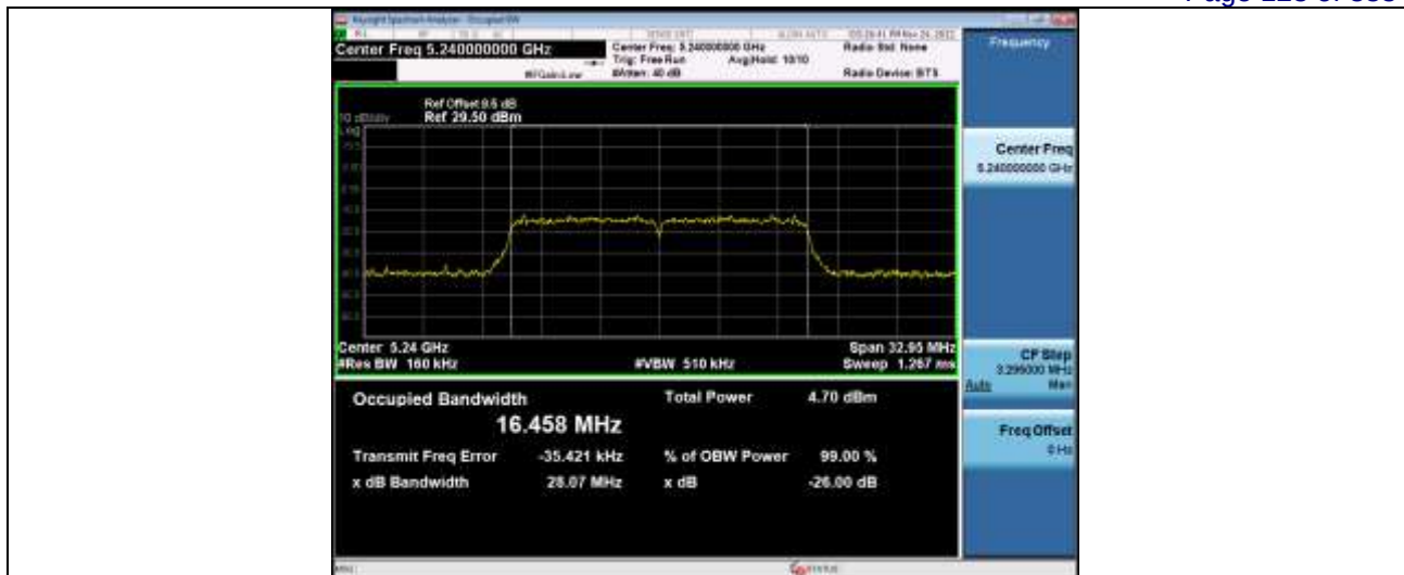
-26dB and 99% Emission Bandwidth 5_2GWiFi NVNT_ANT6 802_11n(HT20) 5180_20M
