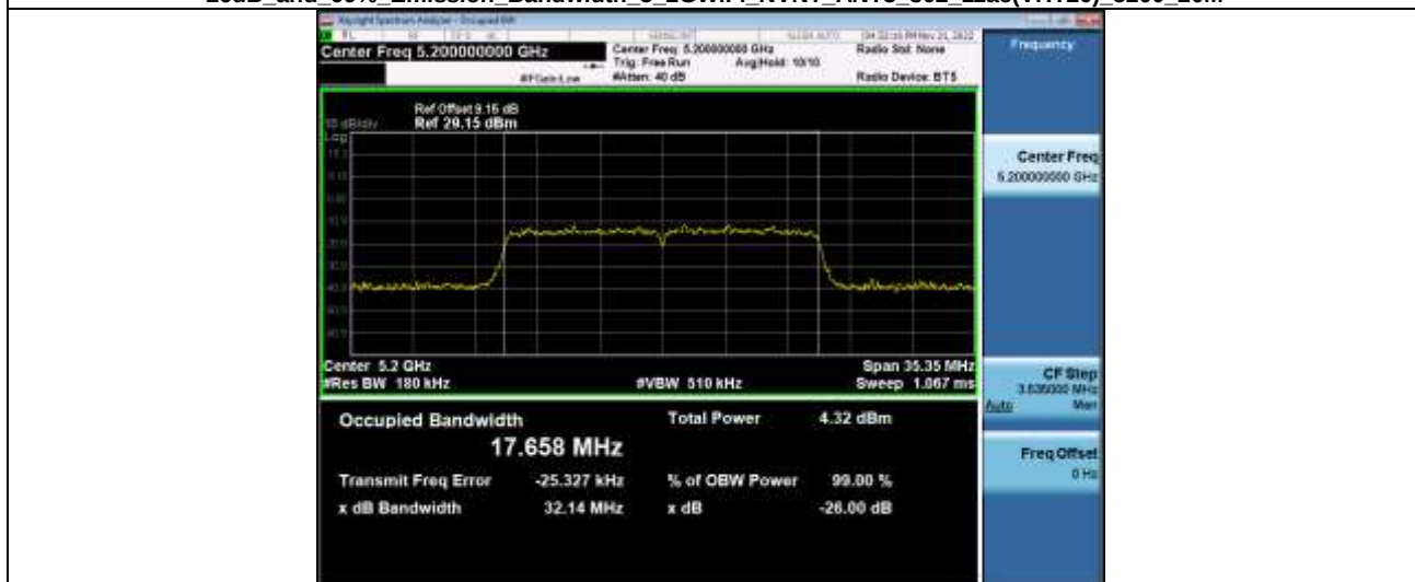
-26dB and 99% Emission Bandwidth 5 2GWiFi_NVNT_ANT3_802_11ac(VHT20)_5240_20M
