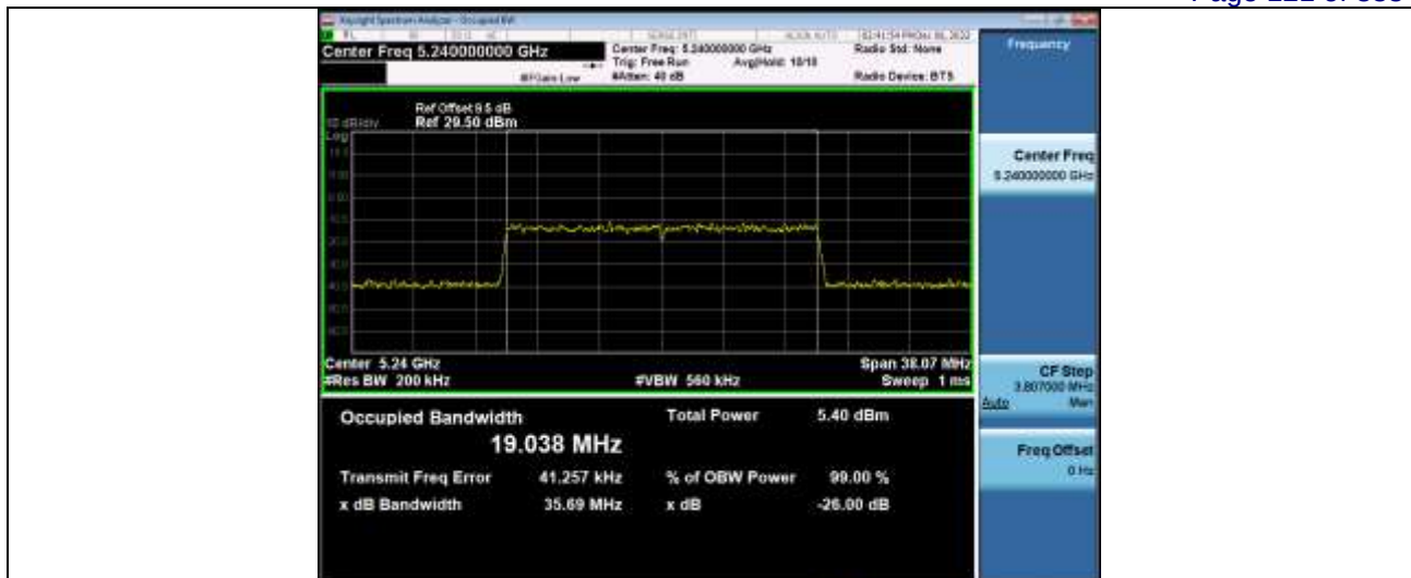
-26dB and 99% Emission Bandwidth 5_2GWiFi_NVNT_ANT5_802_11ax(HE40)_5190_40M
