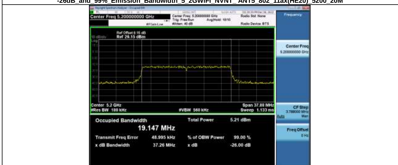
-26dB and 99% Emission Bandwidth 5 2GWiFi NVNT ANT5_802_11ax(HE20) 5240 20M
