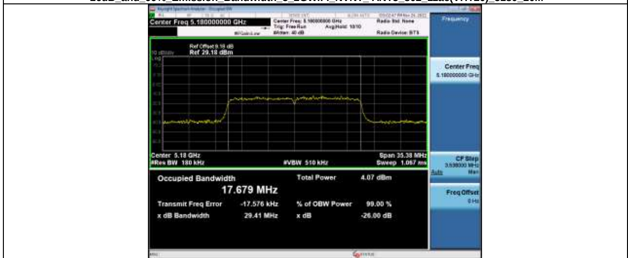
-26dB and 99% Emission Bandwidth 5_2GWiFi_NVNT_ANT5_802_11ac(VHT20)_5200_20M
