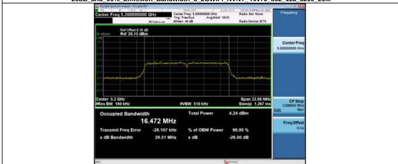
-26dB and 99% Emission Bandwidth 5 2GWiFi NVNT ANT6 802 11a 5200 20M
