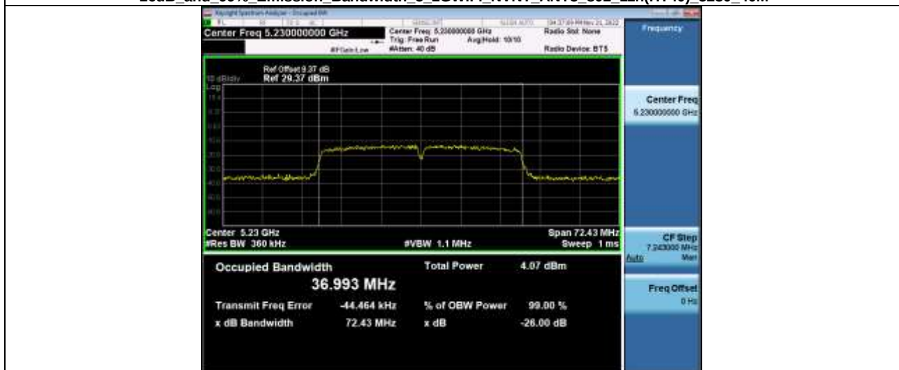
-26dB and 99% Emission Bandwidth 5_2GWiFi_NVNT_ANT3_802_11n(HT40)_5230_40M
