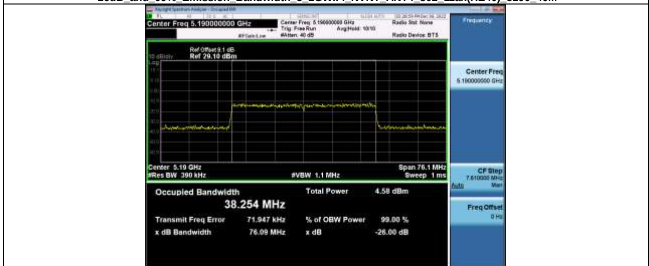
-26dB and 99% Emission Bandwidth 5_2GWiFi_NVNT_ANT4_802_11ax(HE40)_5190_40M
