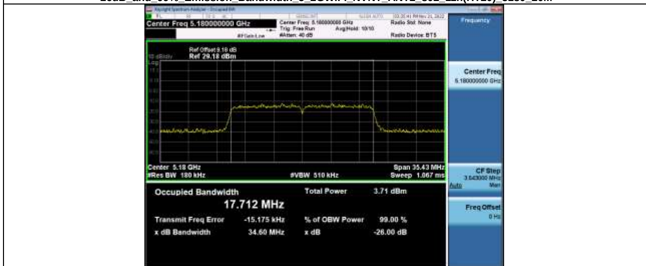
-26dB and 99% Emission Bandwidth 5_2GWiFi_NVNT_ANT2_802_11n(HT20)_5200_20M
