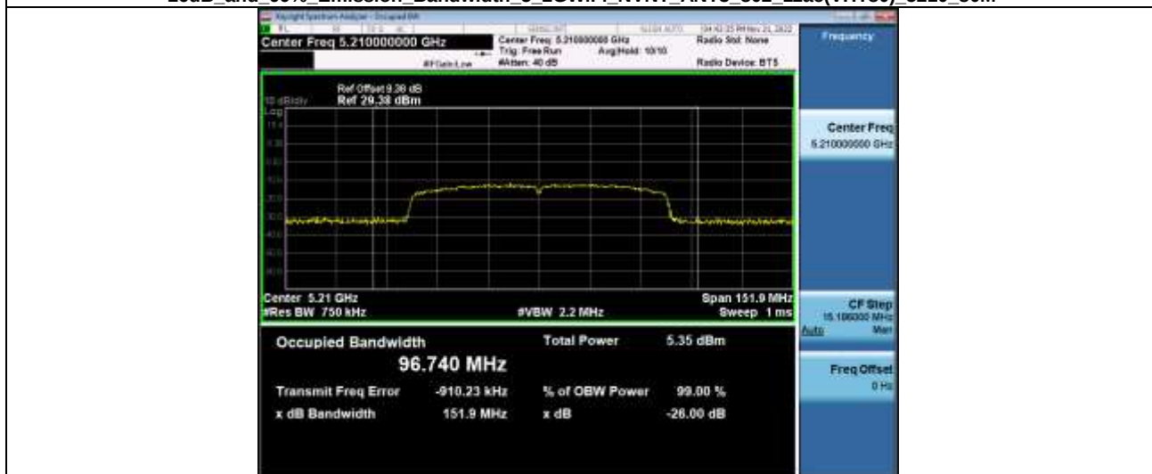
-26dB and 99% Emission Bandwidth 5 2GWiFi NVNT ANT3 802_11ac(VHT80) 5210_80M
