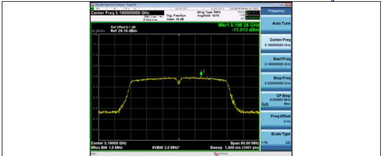
Power Spectral Density 5_2GWiFi_802_11n(HT40)_5230_40M
