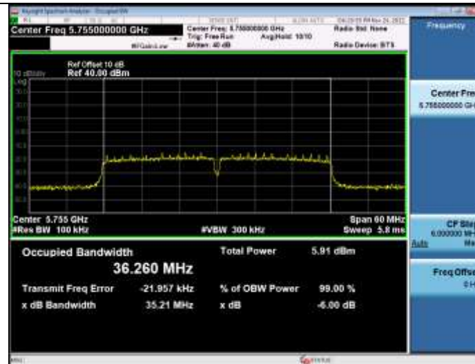
-6dB Emission Bandwidth 5_8WiFi 802_11ac(VHT40)_5795_40M
