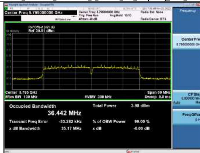
-6dB Emission Bandwidth 5_8WiFi 802_11n(HT40)_5795_40M
