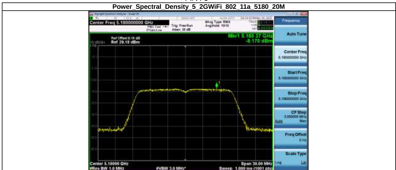
Power Spectral Density 5 2GWiFi 802 11a 5200 20M
