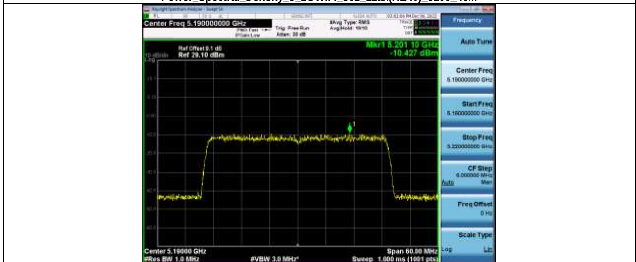
Power Spectral Density 5_2GWiFi_802_11ax(HE40)_5230_40M
