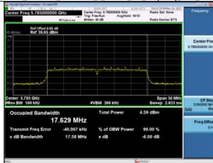
-6dB Emission Bandwidth 5.8GHz WiFi 802.11n(HT20) 5785_20M
