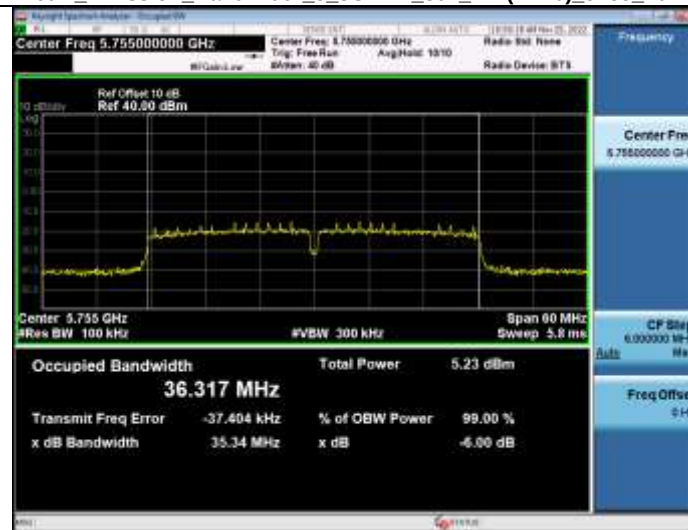
-6dB Emission Bandwidth 5_8WiFi 802_11n(HT40)_5755_40M
