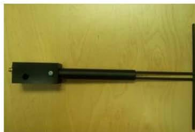
Figure 1 – MVG COMOSAR Validation Dipole
