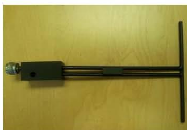
Figure 1 – MVG COMOSAR Validation Dipole
