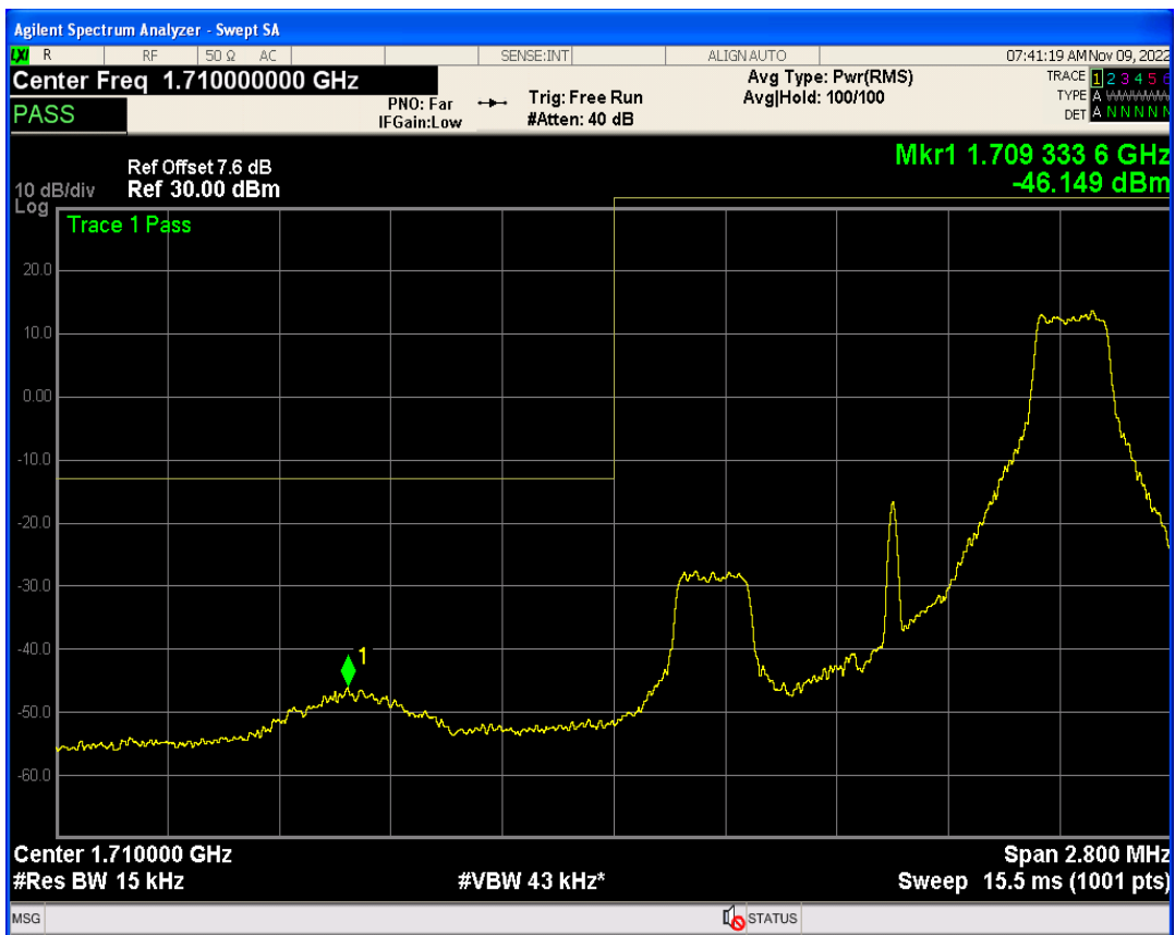
Band4 QPSK BW=1.4MHz Channel=20393 RB Size=1 Position=#0
