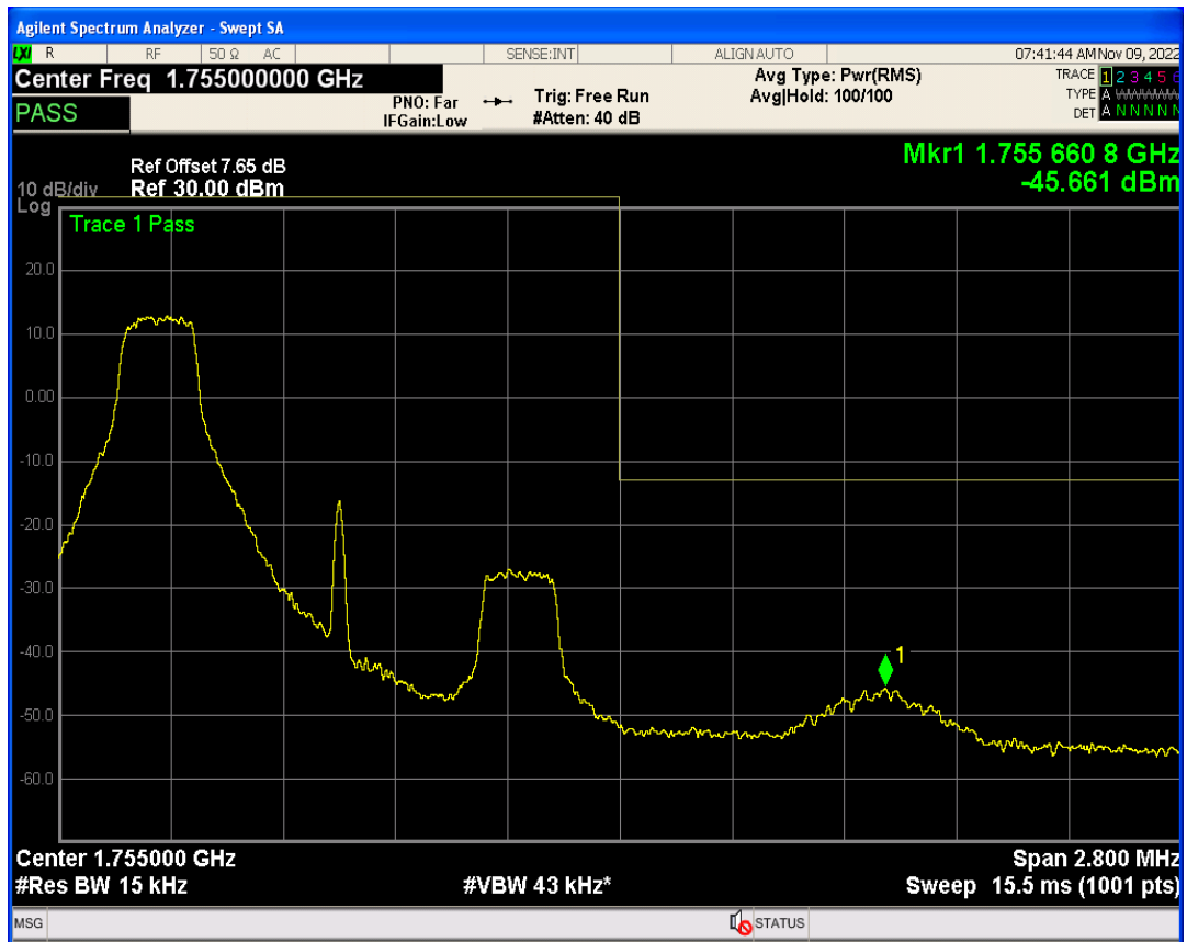
Band4 QAM16 BW=1.4MHz Channel=20393 RB Size=1 Position=#Max
