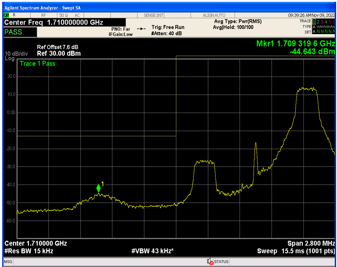
Band66 QAM16 BW=1.4MHz Channel=131979 RB Size=1 Position=#0
