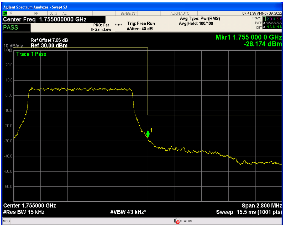
Band4 QAM16 BW=1.4MHz Channel=20393 RB Size=1 Position=#0
