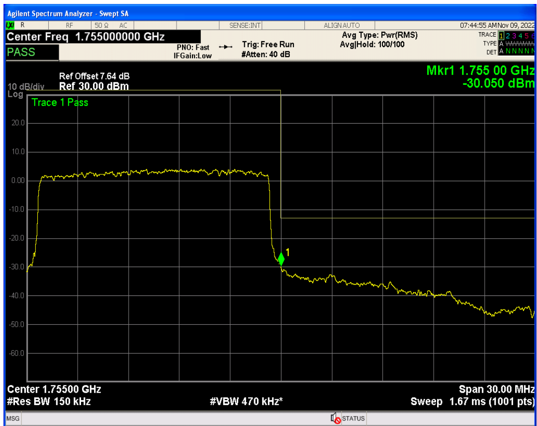
Band4 QAM16 BW=15MHz Channel=20325 RB Size=1 Position=#Max
