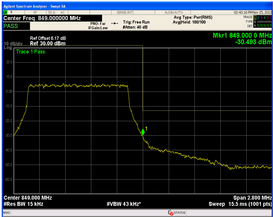
Band5 QAM16 BW=1.4MHz Channel=20643 RB Size=1 Position=#Max
