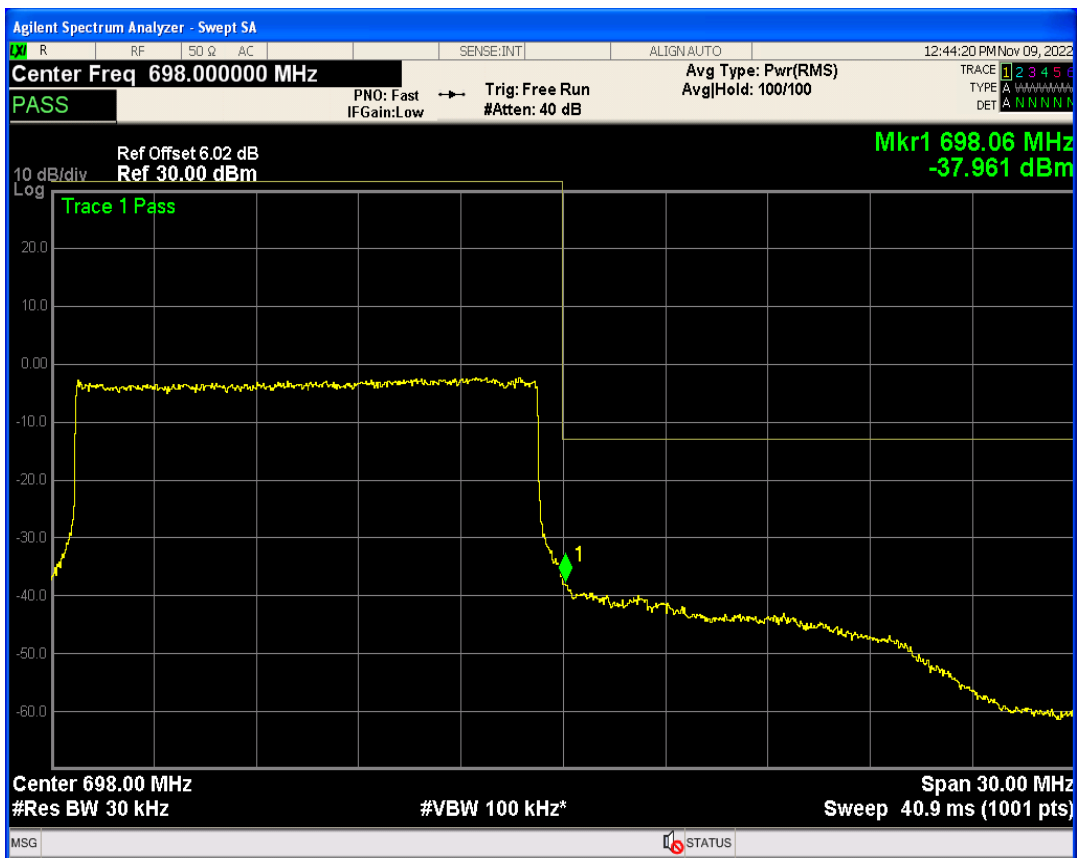
Band71 QAM16 BW=15MHz Channel=133397 RB Size=1 Position=#0
