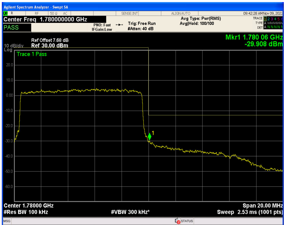
Band66 QAM16 BW=10MHz Channel=132622 RB Size=1 Position=#0
