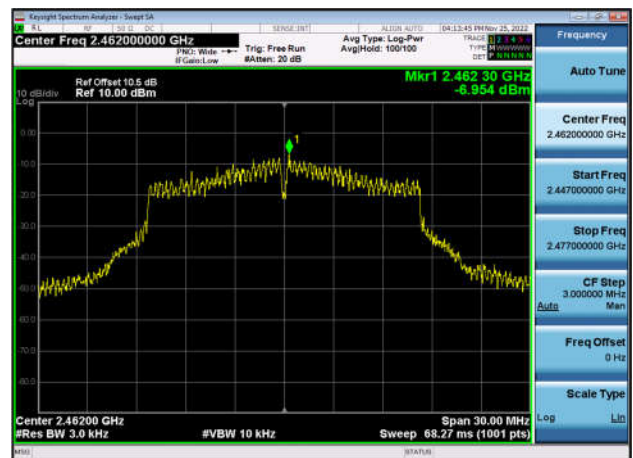
Power spectral density-802.11g ,2462MHz,Ant0
