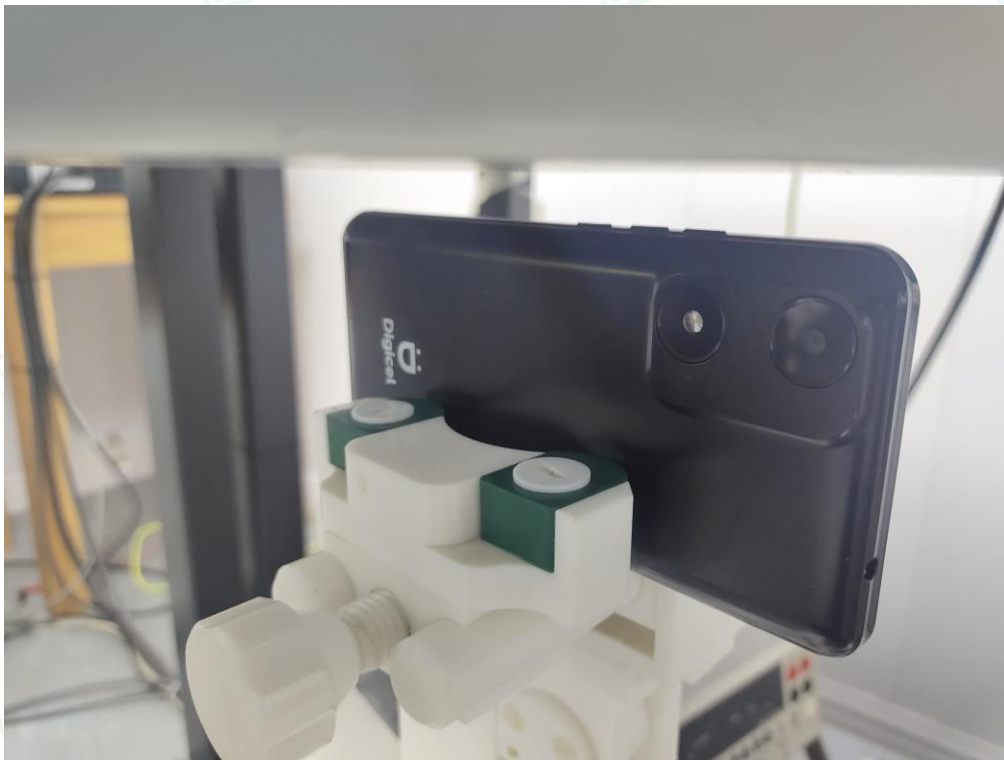
10mm body-worn Right Side Setup Photo (hotspot)
