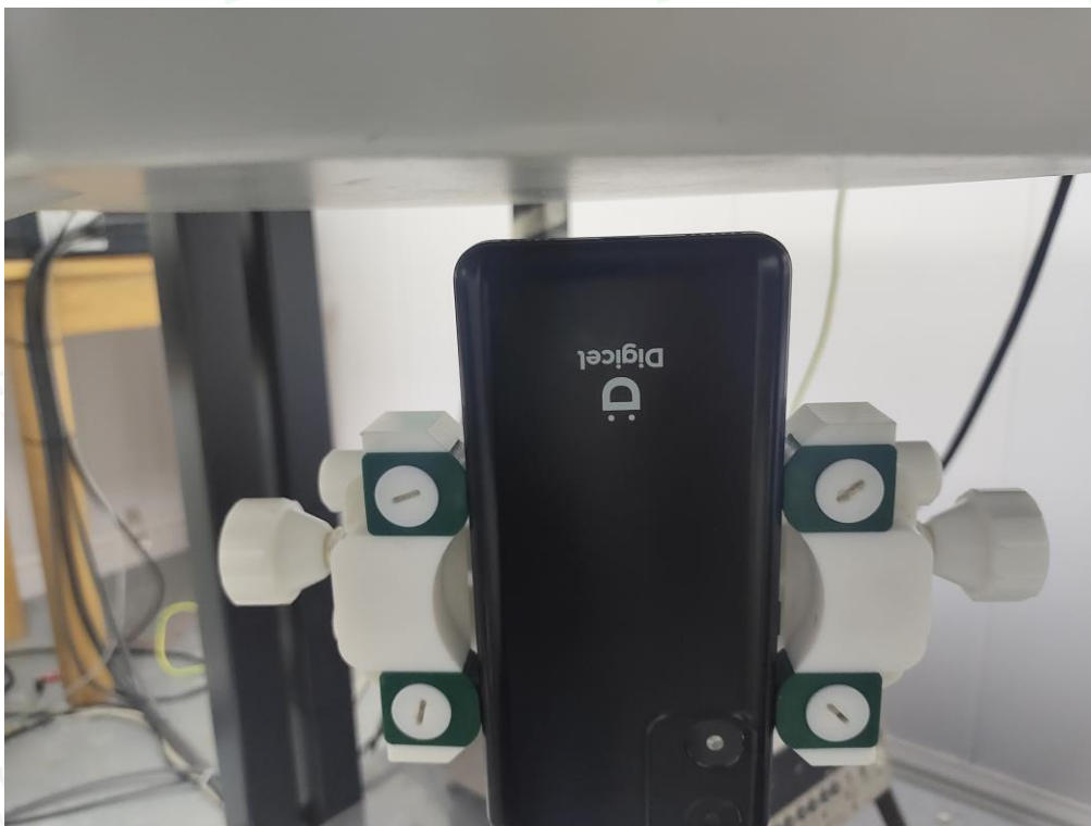
10mm body-worn Bottom Side Setup Photo (hotspot)
