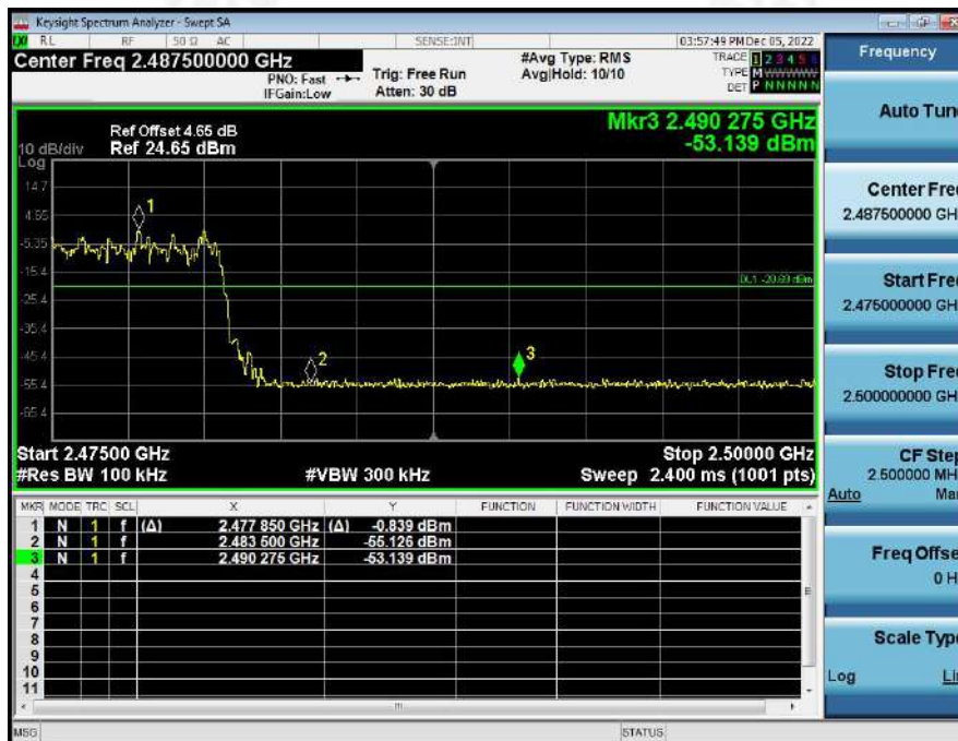
\pi/4 -DQPSK Hopping Band edge-right side
