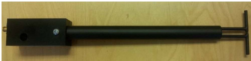
Figure 1 – MVG COMOSAR Validation Dipole
