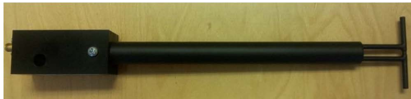
Figure 1 – MVG COMOSAR Validation Dipole
