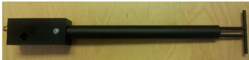
Figure 1 – MVG COMOSAR Validation Dipole
