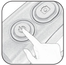
Long press the on button to switch on Recorder indicator blue light
