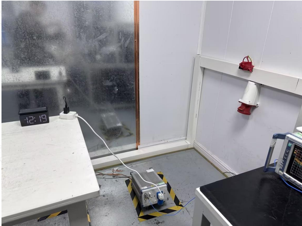
Conducted Emission-AC charge mode
