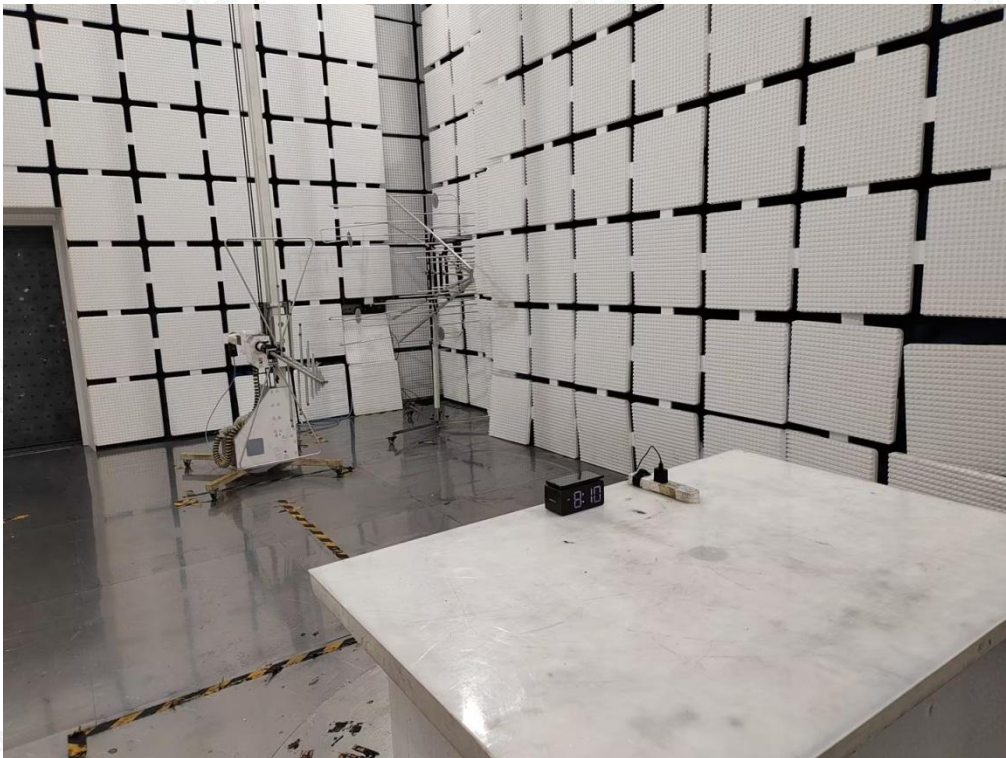
Radiated Emission below 1GHz
