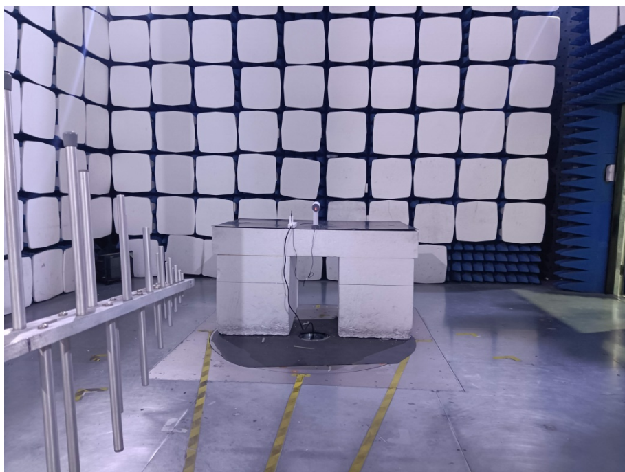
Radiation Emission Test Setup (30MHz to 1GHz)
