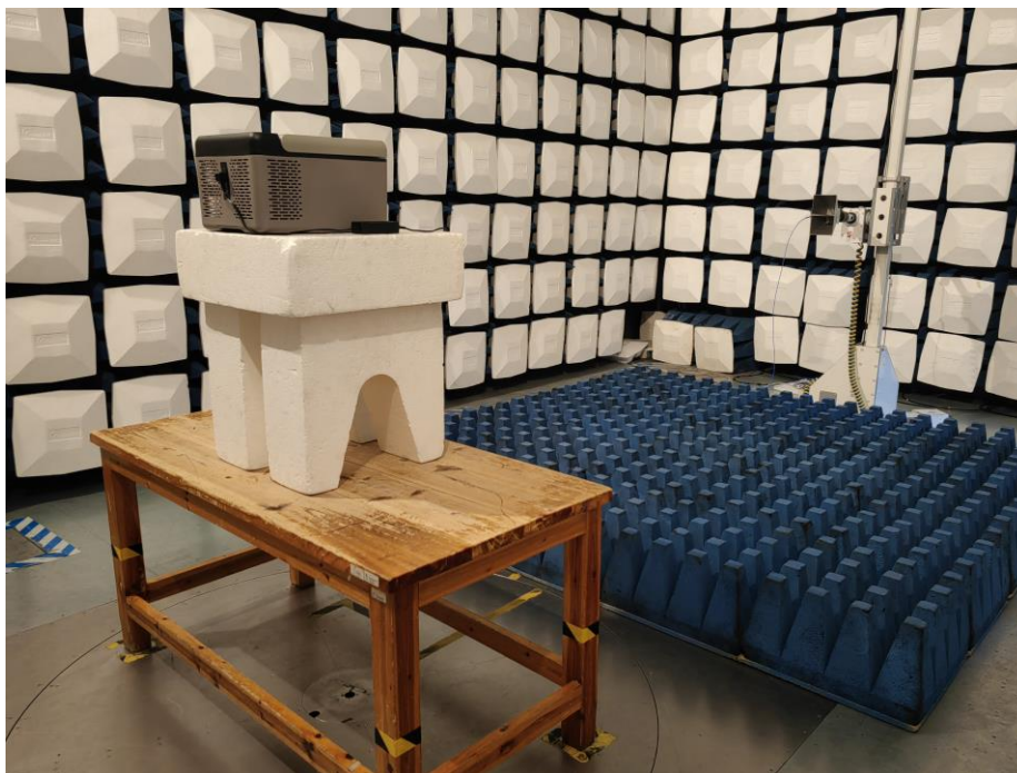
Test Setup For Radiated Emission (Above 1GHz)
