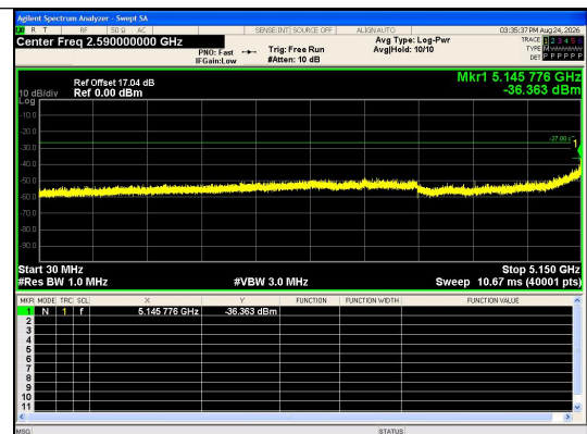
Spurious Emission: 30.0~5150 MHz IEEE 802.11a Channel 36 20MHz Antenna 0
